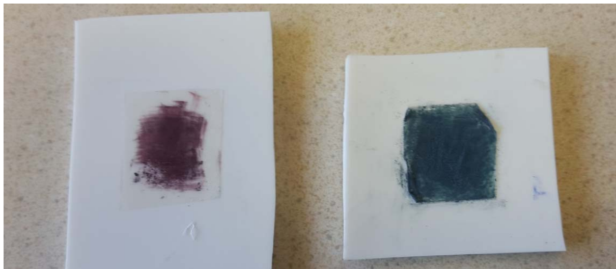
Figure S28. Sample mounting method used for collection of the solid-state visible reflectance spectra. The sample on the left is 1 after drying at 403 K under a N_2(g) flow. The sample on the right was initially treated in the same way, then exposed to THF vapour for 4 hours to regenerate 1 ·THF (shown) - this is the sample that was used to give the blue, pink and green lines in Figure S19.
