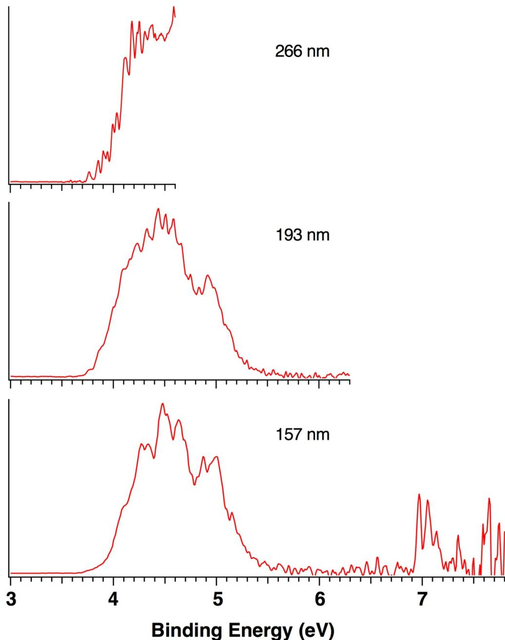
**Figure S1.** The 20 K NIPE spectra of  $\text{P}_2\text{N}_3^-$  at 266, 193, and 157 nm, respectively.
