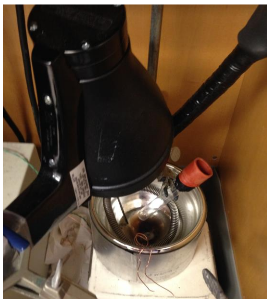
Figure S1. Representative reaction set-up using a 100-W Hg lamp. Ice is excluded for clarity.
