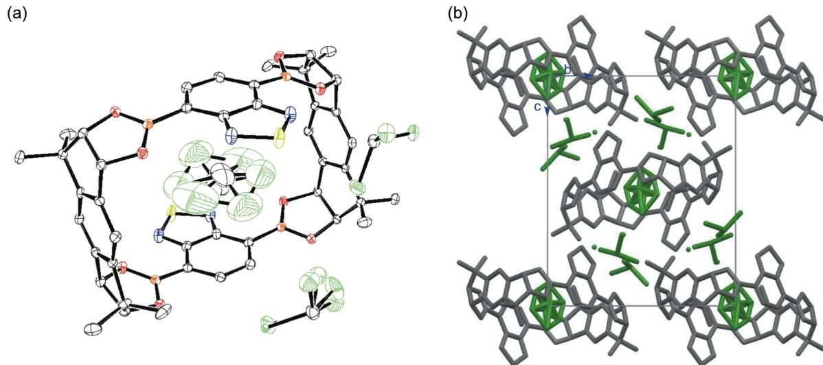
**Figure S31. X-ray crystal structure of **3•CHCl<sub>3</sub>•4CHCl<sub>3</sub>** (CCDC 1005497).** All hydrogen atoms are omitted for clarity. (a) ORTEP structure with thermal ellipsoids shown at 50% probability (C = gray, O = red, B = orange, N = blue, S = yellow, Cl = green). (b) Schematic representation of the unit cell structure viewed along *a*-axis (**3** = gray, chloroform = green).
