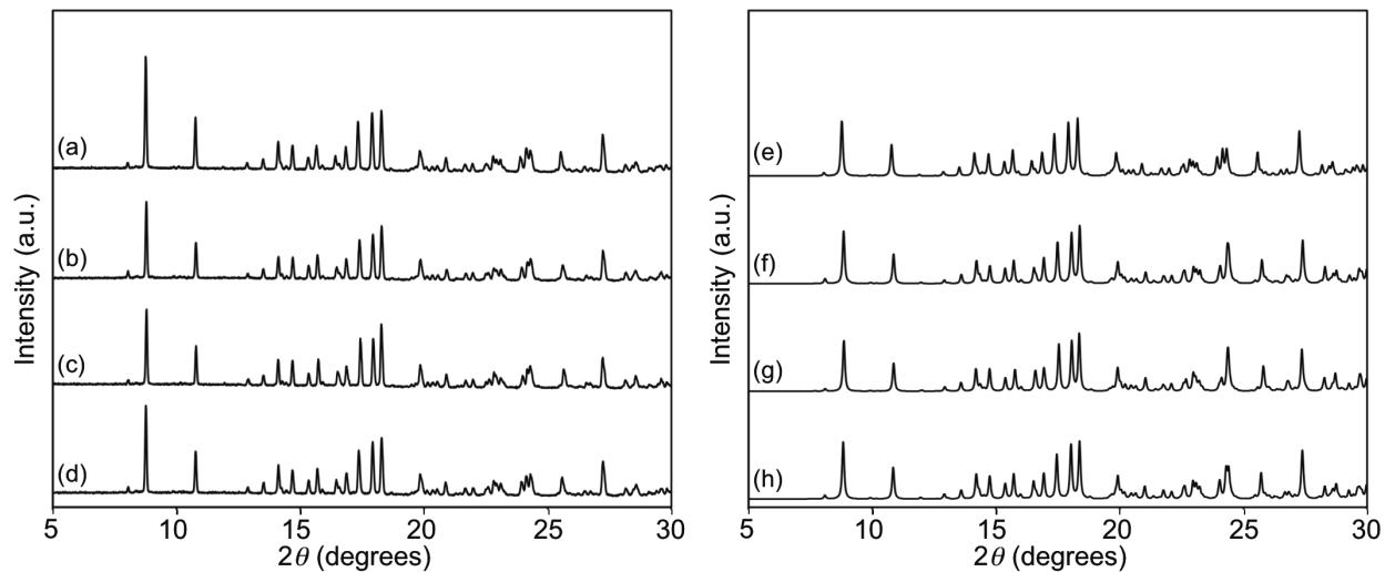
**Figure S27.** (a)~(d) Experimental PXRD patterns of the precipitate of (a) **3•NA•4CHCl<sub>3</sub>**, (b) **3•BT•4CHCl<sub>3</sub>**, (c) **3•BF•4CHCl<sub>3</sub>**, (d) **3•QU•4CHCl<sub>3</sub>**. (e)~(h) Simulated PXRD pattern calculated from the single-crystal structure of (e) **3•NA•4CHCl<sub>3</sub>**, (f) **3•BT•4CHCl<sub>3</sub>**, (g) **3•BF•4CHCl<sub>3</sub>**, (h) **3•QU•4CHCl<sub>3</sub>**.
