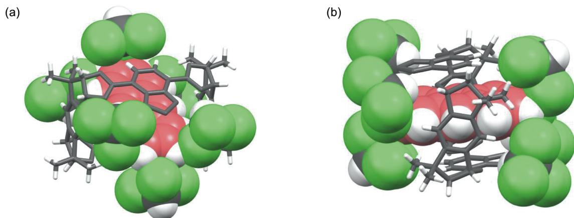
**Figure S35.** Virtual schematic representation of **3**•ANT•4CHCl<sub>3</sub> in *P*2<sub>1</sub>/*c* crystal structure. Included anthracene molecule and chloroform molecules are shown as space-filling model, and **3** is represented as stick model. (a) Top view. (b) Side view.
