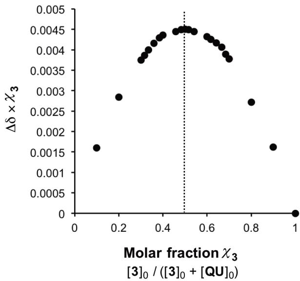
**Figure S10.** Job plot for NMR titration data of **3** and **QU**.
