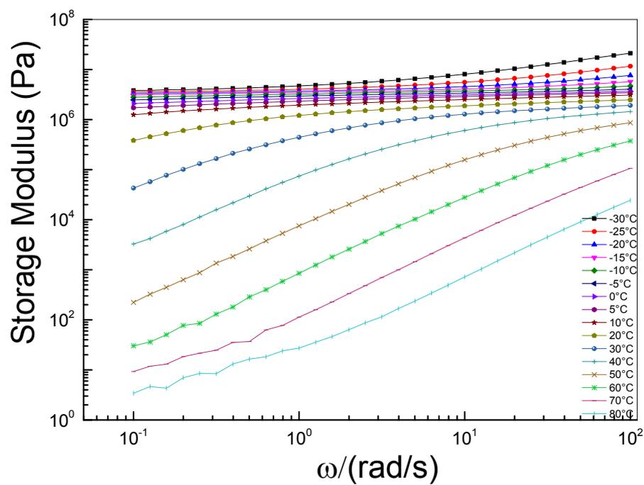
**Figure S4.** Frequency sweep for supramolecular polyurethane **1** at different temperatures. Isothermal frequency sweep data obtained at frequencies between 0.1 and 100  $\text{rad s}^{-1}$  and at 5  $^{\circ}\text{C}$  intervals between -30 and 10  $^{\circ}\text{C}$  and 10  $^{\circ}\text{C}$  intervals between 10 and +80  $^{\circ}\text{C}$ .
