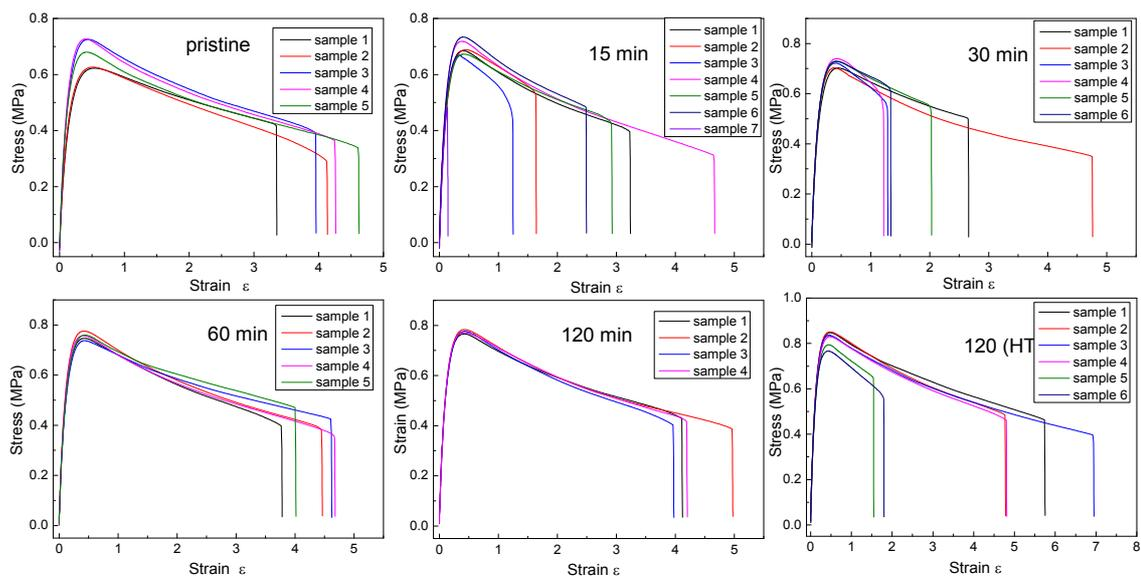
**Figure S5.** The stress-strain curves for pristine and healed polyurethane **1**. Pristine) pristine polyurethane **1** without any heat treatment, 15 min) healing after 15 minutes, 30 min) healing after 30 minutes, 60 min) healing after 60 minutes, 120 min) healing after 120 minutes, 120 min (HT)) heat treated pristine polyurethane **1** at 37 °C for 120 minutes. The ends of the curves represent specimen failure.
