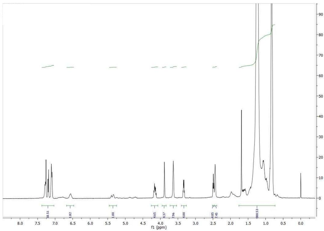
**Figure S1.**  $^1\text{H}$  NMR of polyurethane **1** in  $\text{CDCl}_3$  at  $25\text{ }^\circ\text{C}$
