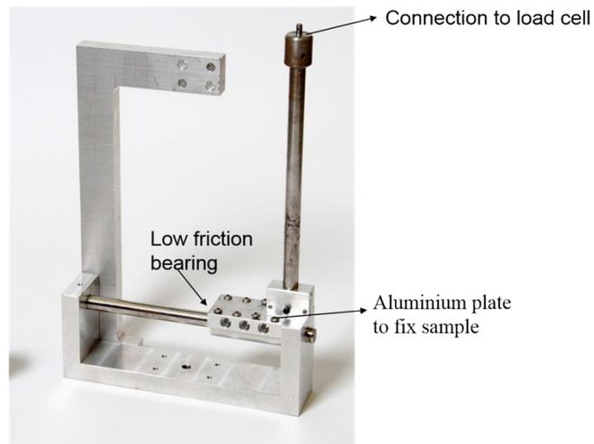
**Peel test loading rig**
