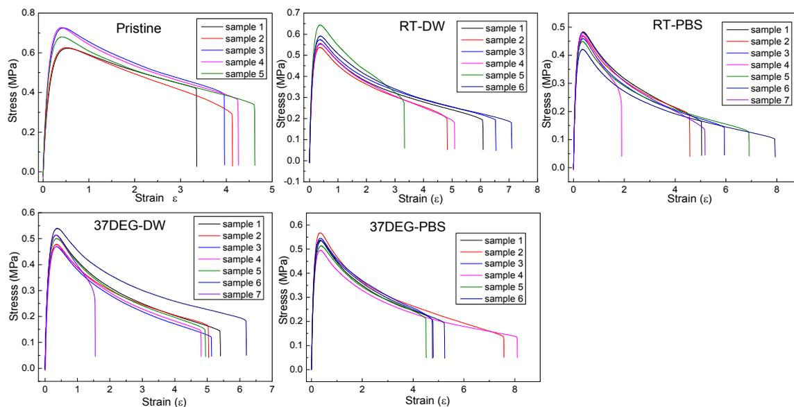
**Figure S6.** The stress-strain curves for pristine polyurethane **1** under different physiological conditions. Pristine) pristine polyurethane **1**, RT-DW) room temperature in distilled water for 48 hours, RT-PBS) room temperature in PBS solution for 48 hours, 37 DEG-DW) 37 °C in distilled water for 12 hours, 37 DEG-PBS) 37 °C in PBS solution for 12 hours. The ends of the curves represent specimen failure.
