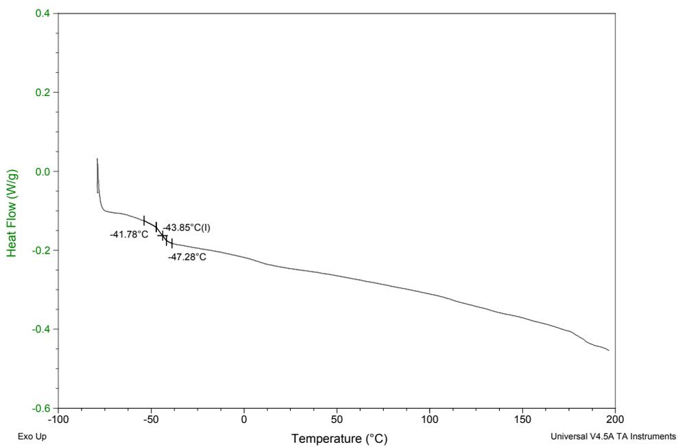
**Figure S3.** DSC thermogram of polyurethane 1
