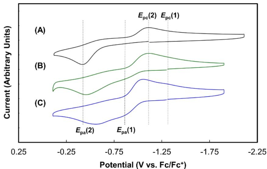
**Figure S17.** Normalized cyclic voltammograms of **1–Ce** of different optical purities (A) 100% ee (black trace) (B) 50% ee (green trace) (C) 0% ee (blue trace). Cyclic voltammetry performed in THF ( $[Ce] = \sim 1$  mM; THF,  $[NPr_4][BAr^F] = 0.100$  M,  $v = 500$  mV·s $^{-1}$ ). Dashed lines provided as a guide for the eye to identify  $E_{pa}$  and  $E_{pc}$ .
