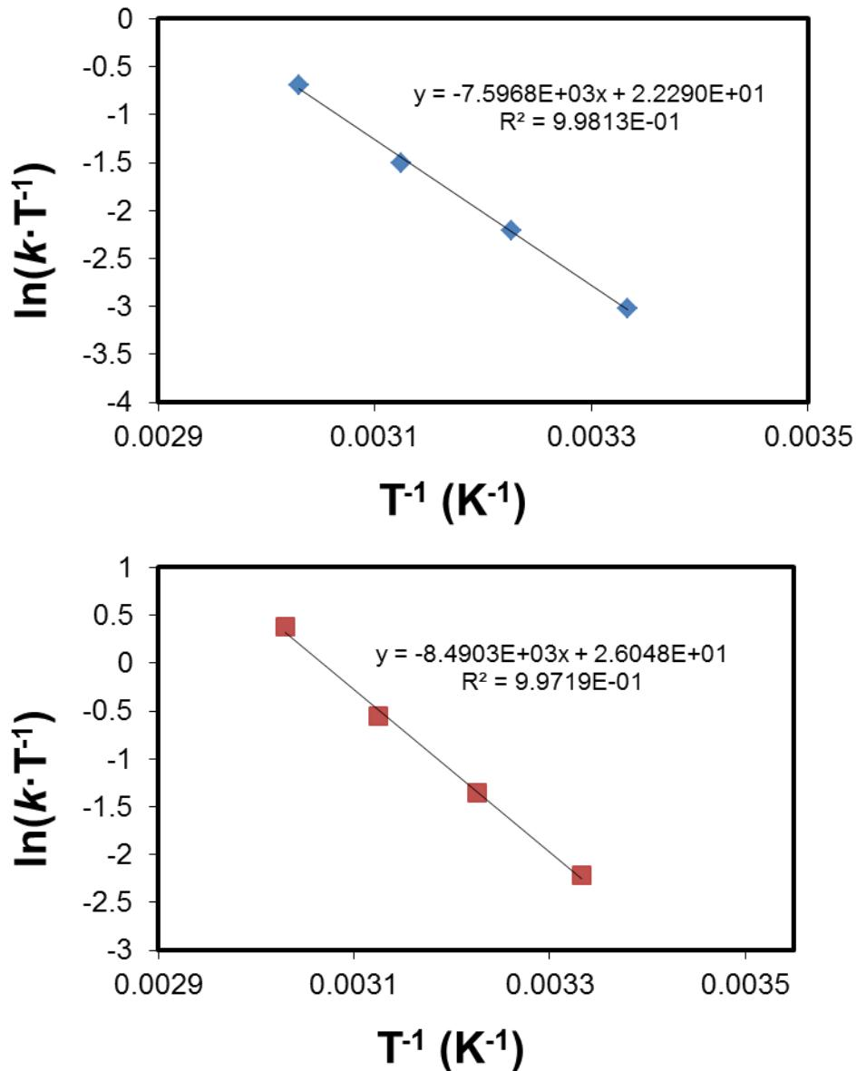
**Figure S14.** Eyring plots (*top* = Li<sub>A</sub> → Li<sub>B</sub>, *bottom* Li<sub>B</sub> → Li<sub>A</sub>) obtained from 2D-EXSY <sup>7</sup>Li-NMR experiments of **1-Yb(het)** (19.3 mM) taken at 300, 310, 320, and 330 K (t<sub>mix</sub> = 5 ms).
