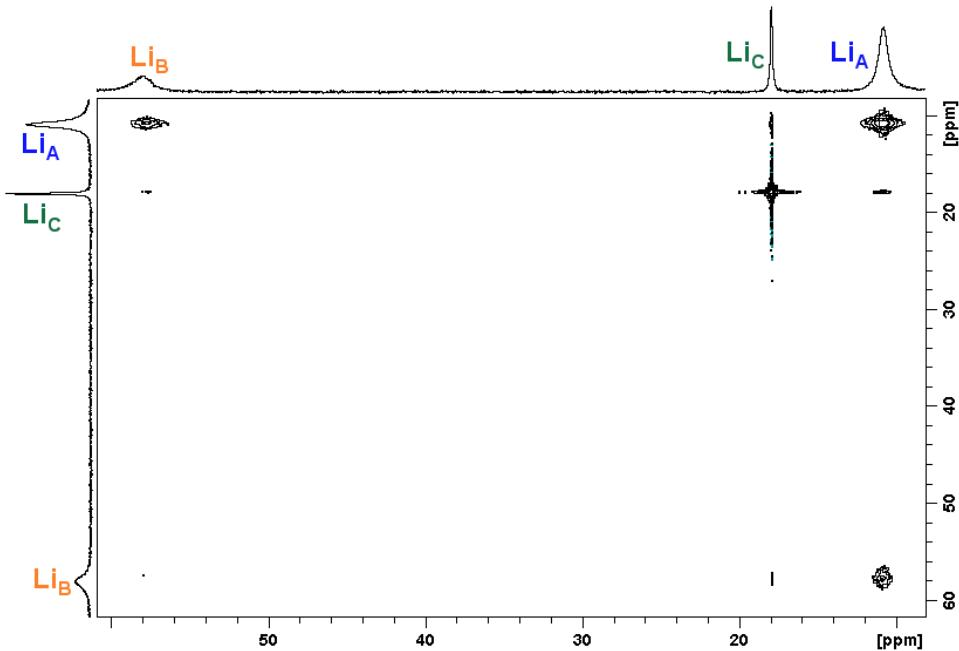
**Figure S15.** 2D <sup>7</sup>Li-NMR EXSY experiment of **1-Ce(het) / 1-Ce(homo)** ([Ce] = 24.4 mM;  $t_{mix}$  = 10 ms, 315 K; **1-Ce** = 0% ee) taken in THF-*d*<sub>8</sub>.
