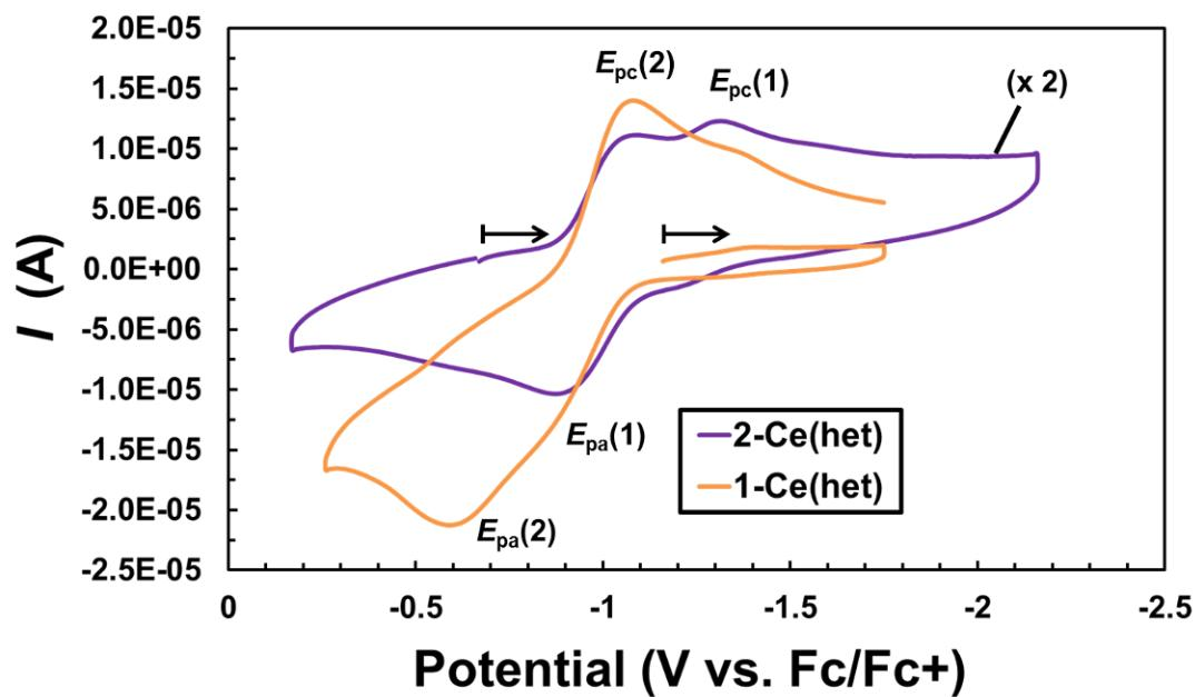
**Figure S19.** Overlay of cyclic voltammograms for  $[\text{Li}_2(\text{THF})_4][\text{BINOLate}]_3\text{Ce}$  (**2-Ce(het)**) and  $[\text{Li}_3(\text{THF})_6][\text{BINOLate}]_3\text{Ce}$  (**1-Ce(het)**) (**1-Ce** = 0% ee) collected at  $250 \text{ mV}\cdot\text{s}^{-1}$
