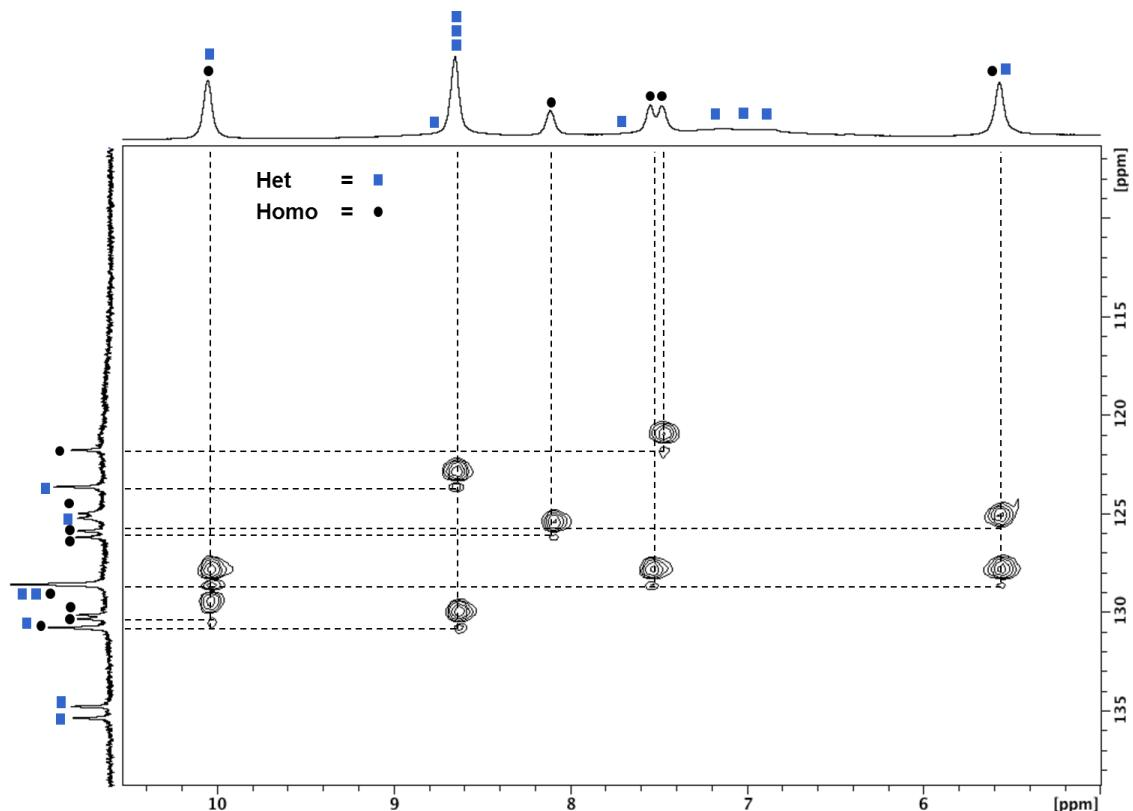
**Figure S6.**  $^1\text{H}$ - $^{13}\text{C}$  HSQC-NMR spectrum (500 MHz, THF- $d_8$ ) of **1-Ce(het)** (**1-Ce** = 0% ee). Dashed lines provided a guide for the eye to identify cross peaks. ■ = **1-Ce(het)**, ♦ = **1-Ce(homo)**.
