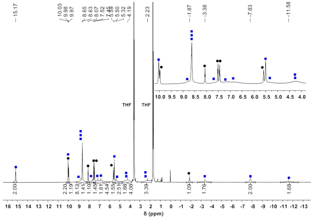
**Figure S4a.**  $^1\text{H}$ -NMR(500 MHz, THF- $d_8$ ) of 1-Ce(het). ■ = 1-Ce(het), ♦ = 1-Ce(homo).
