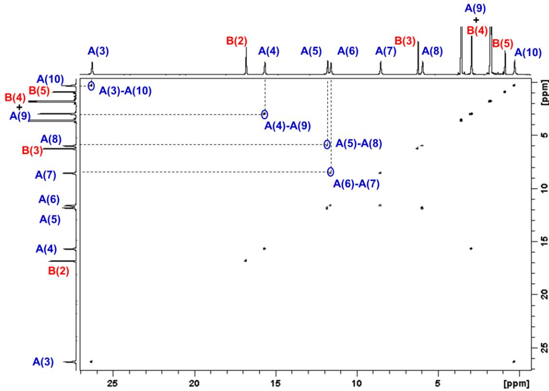
**Figure S12.** Representative 2D <sup>1</sup>H-NMR EXSY experiment of **1**-Yb(het) (19.3 mM;  $t_{\text{mix}} = 5$  ms, 300 K; **1**-Yb = 0% ee) taken in THF-*d*<sub>8</sub>.
