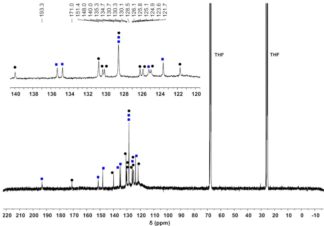
**Figure S4b.**  $^{13}\text{C}\{^1\text{H}\}$ -NMR(126 MHz, THF- $d_8$ ) of 1-Ce(het). ■ = 1-Ce(het), ♦ = 1-Ce(homo).
