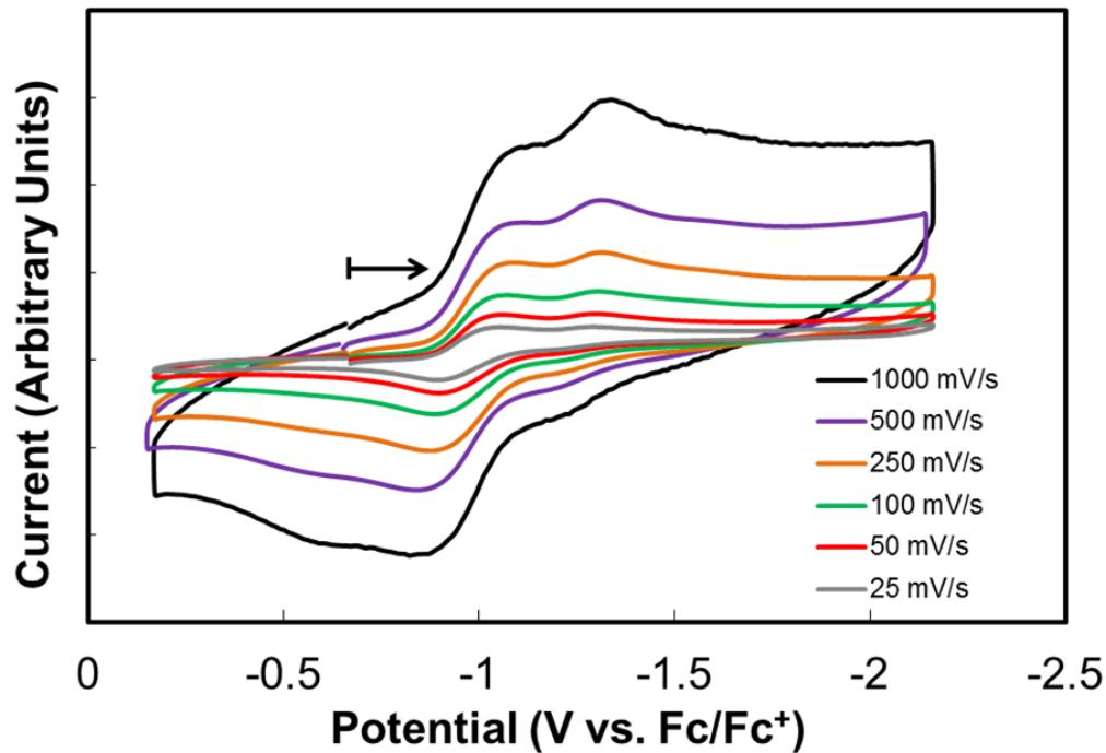
**Figure S18.** Cyclic voltammogram for  $[\text{Li}_2(\text{THF})_4][\text{BINOLate}]_3\text{Ce}$  (**2-Ce(het)**) (**2-Ce** = 0% ee) collected from  $-0.17$  to  $-2.16$  V
