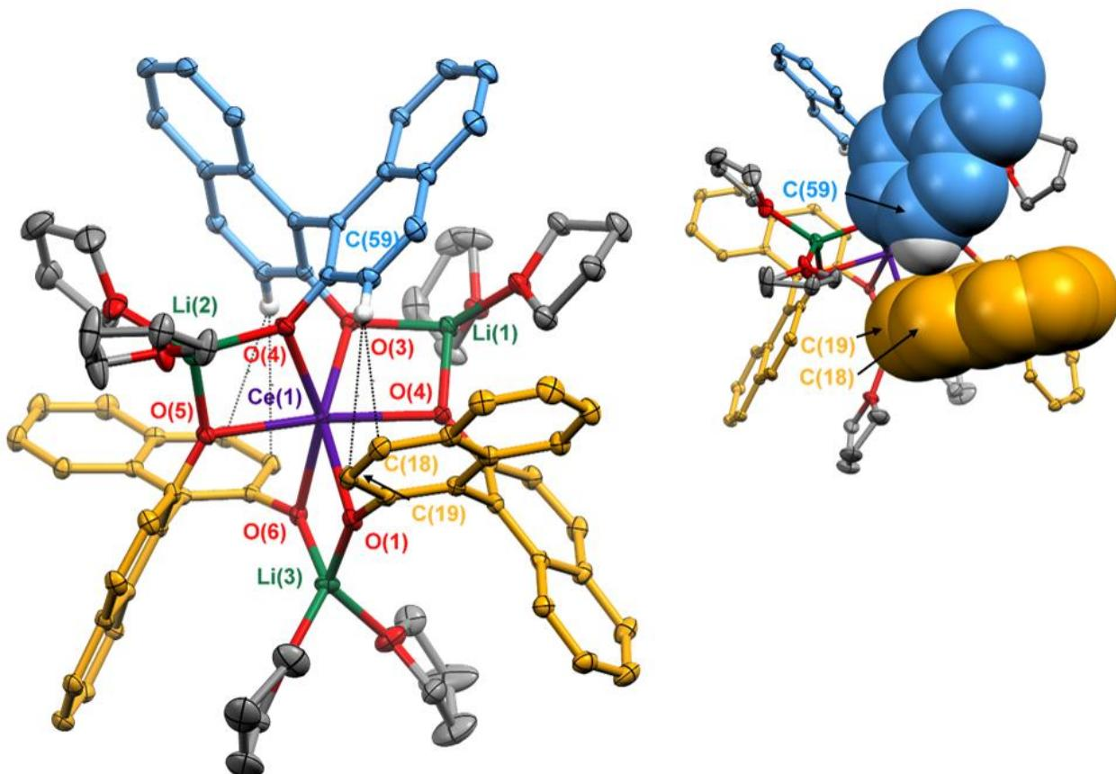
**Figure S21.** Thermal ellipsoid plot (30% probability) and space-filling model of **1–Ce(het)** highlighting C–H–π interaction in the solid state. The BINOLate ligands have been colored blue and yellow to indicate the SS/RR and R/S fragments respectively.
