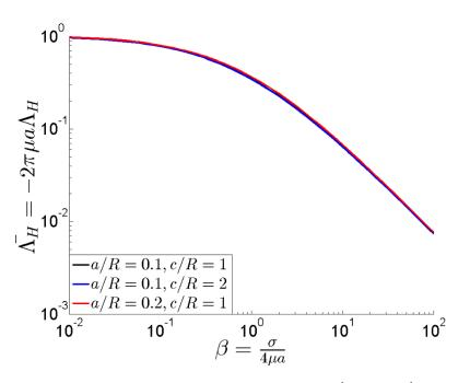
From the plot shown above, it can be seen that different value of c/R and a/R result in almost same  $\overline{\Lambda_H} - \beta$  curve. This curve can be fitted by:
