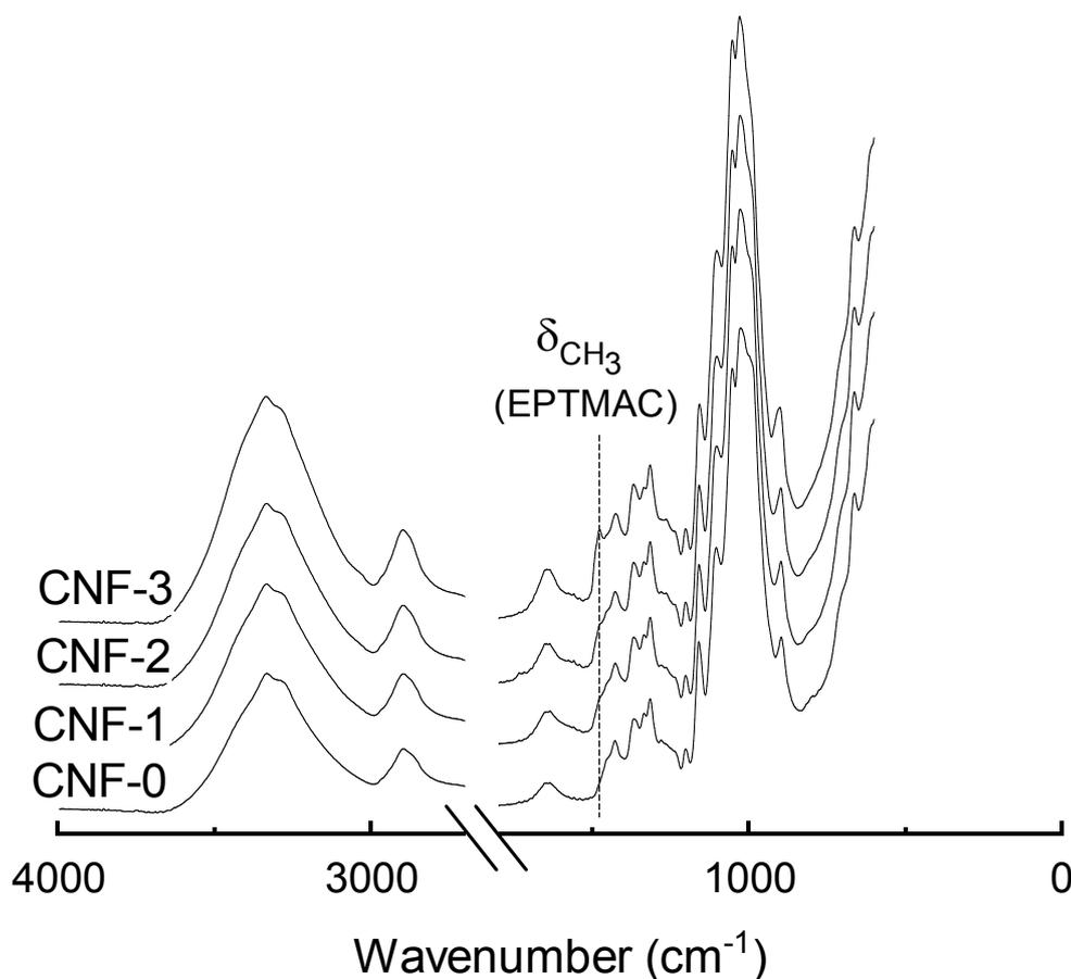
Figure 1 : FTIR spectra of unmodified nanofibers (CNF-0) and cationic nanofibers (CNF-1; CNF-2; CNF-3). A peak corresponding to the bending vibration of the methyl moieties of the quaternary ammonium groups could be seen for CNF-3 while a shoulder is observed for CNF-1 and CNF-2.
