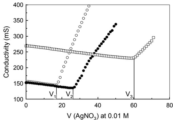
Figure 2 : Conductometric titration of ammonium groups in cationic nanofibers.  $V_1$ ,  $V_2$  and  $V_3$  correspond to the volume of silver nitrate needed to titrate 0.5 g of CNF<sub>1</sub>, CNF<sub>2</sub> and CNF<sub>3</sub>, respectively.
