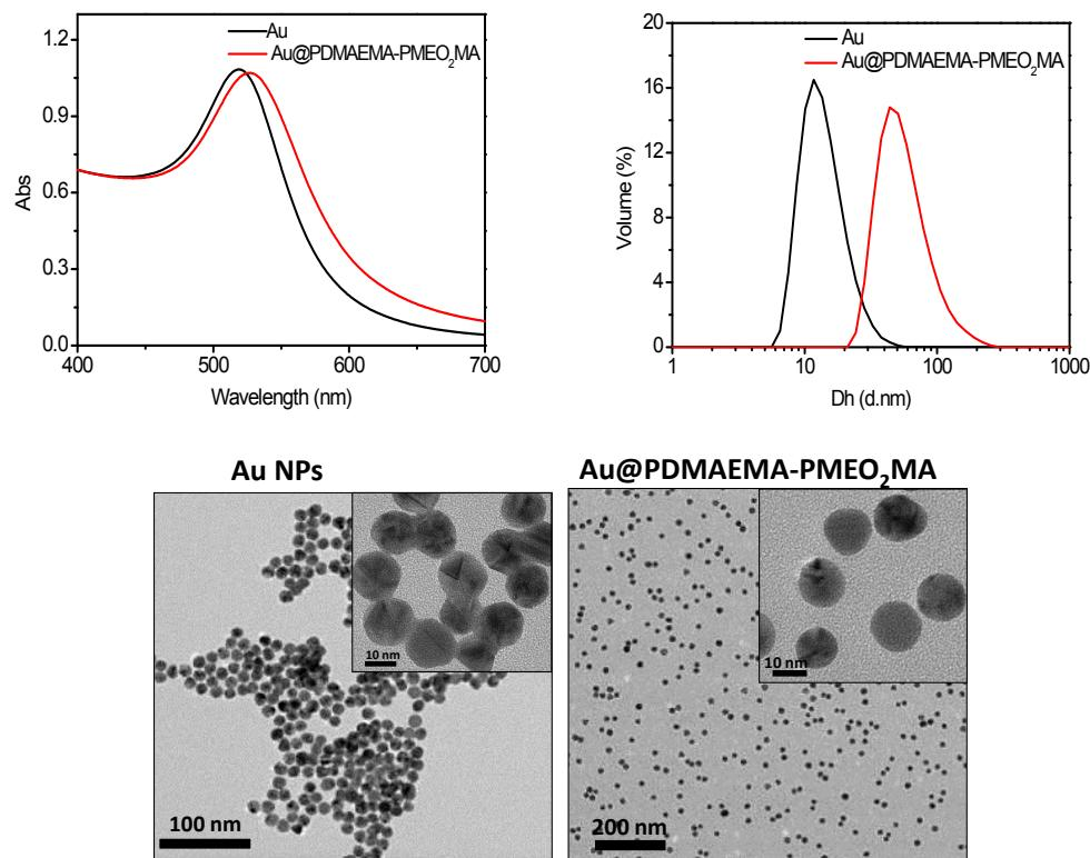
**Figure S3. UV–vis spectra, size distributions and TEM images of Au NPs and Au@PDMAEMA<sub>27</sub>-b-PMEO<sub>2</sub>MA<sub>80</sub> particles dispersed in aqueous solutions.**
