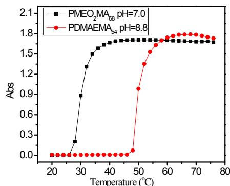
**Figure S2. Thermal profile of PMEO<sub>2</sub>MA (black) and PDMAEMA (red) in aqueous solutions as probed by UV–vis spectra.**
