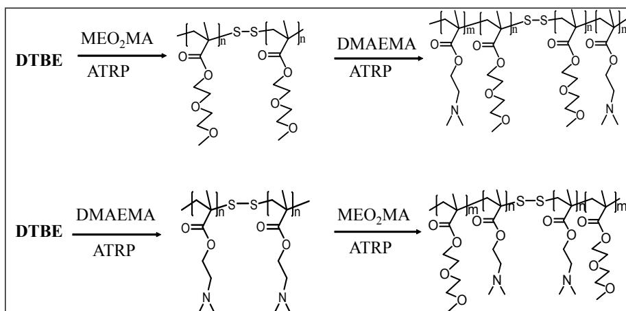
Scheme 2. Synthesis of the PDMAEMA-b-PMEO<sub>2</sub>MA-b-PDMAEMA, PMEO<sub>2</sub>MA-b-PDMAEMA-b-PMEO<sub>2</sub>MA triblock copolymers.
