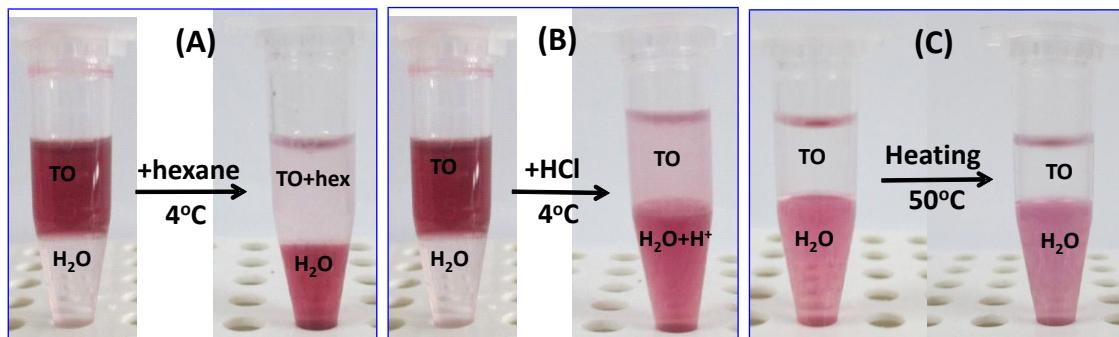
**Figure S6.** Photographs of the phase transfer process for the Au@PMEO<sub>2</sub>MA<sub>34</sub>-b-PDMAEMA<sub>46</sub> system: (A) solvent-triggered NP transfer from toluene to the aqueous phase at 4 °C after shaking, (B) acid-triggered NP transfer from toluene to the aqueous phase at 4 °C after shaking, and (C) retention of NPs in the aqueous phase (0.2 M NaCl) upon heating to 50 °C after shaking.
