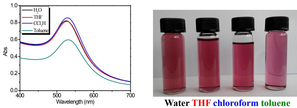
**Figure S4.** Au@PMEO<sub>2</sub>MA<sub>34</sub>-b-PDMAEMA<sub>46</sub> nanoparticles well-dispersed in different solvents (water, THF, chloroform and toluene).
