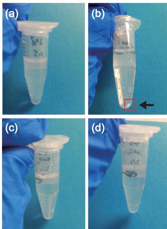
Figure S2. Optical images of PEC aged for 24hs. 20 mol% PDAC, 0.5 M NaCl (upper panel) before (a) and after (b) centrifugation. 50 mol% PDAC, 3.0 M NaCl (lower panel) before (c) and after (d) centrifugation. Centrifugation parameters: 8500 rpm, 15 min. The black arrow and red square help to observe the white precipitate of complex.
