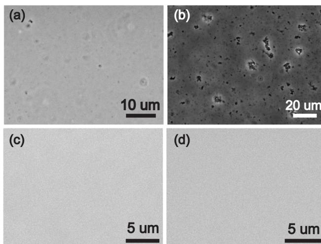
Figure S3. Optical microscope images of PECs aged for 24hs. 20 mol% PDAC, 0.5 M NaCl (upper panel) before (a) and after (b) centrifugation. 50 mol% PDAC, 3.0 M NaCl (lower panel) before (c) and after (d) centrifugation.
