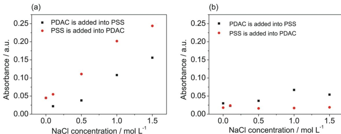
Figure S1. Turbidity of newly prepared complexes with different mixing order. The complex are prepared from (a) 20 mol% PDAC, (b) 80 mol% PDAC, respectively.
