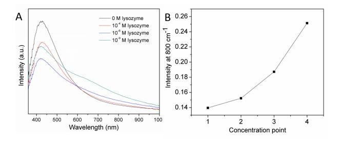
**Figure S1** (A) UV-vis spectra of Ag nanoparticles in presence of different concentrations of lysozyme. (B) The intensity of longitudinal plasmon band at 800 cm<sup>-1</sup> at different concentration points (1-4) of lysozyme which are 0, 10<sup>-4</sup>, 10<sup>-6</sup> and 10<sup>-9</sup> M respectively.
