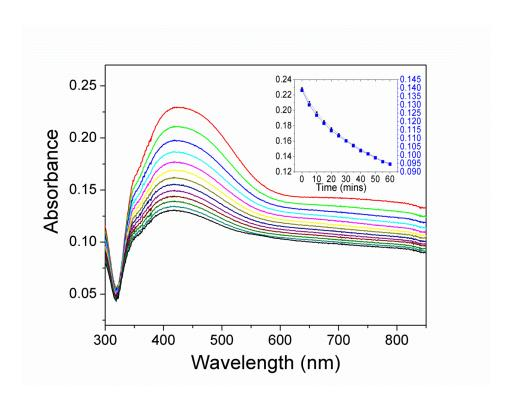
**Figure S2** UV-vis spectra of Ag nanoparticles in presence of 1 M NaCl with intervals of 5 mins between successive spectra. Inset shows the intensity variation of 450 nm and 800 nm peaks.
