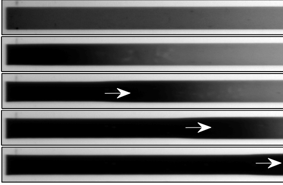
FIG. S1: From top to bottom: zooms on the solidification front at different time scales, channel width w = 150 \mu\text{m} . The snapshots 3, 4 and 5 show the progression of the polymeric solid along the channel (see the white arrows). The channel width is significantly smaller within the dry solid.
