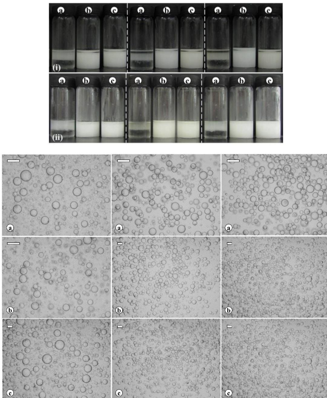
**Figure S5.** (upper) Photographs of glass vials containing 100 cS PDMS-in-(a) sunflower oil, (b) olive oil and (c) rapeseed oil emulsions (1:1, 1 month after preparation) stabilised by different concentrations (given, wt.%) of 75% SiOH fluorinated fumed silica particles. (lower) Corresponding optical micrographs of the emulsions at selected particle concentrations (given, wt.%). Scale bar = 100  $\mu$ m.
