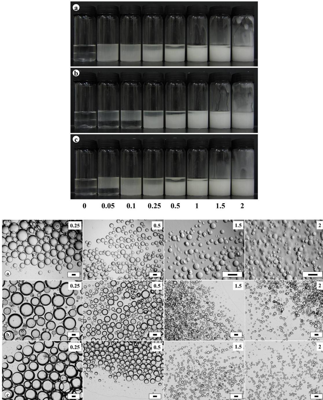
**Figure S6.** (upper) Photographs of glass vials containing (a) sunflower oil-, (b) olive oil-, (c) rapeseed oil-in-20 cS PDMS emulsions (1:1, 1 month after preparation) stabilised by different concentrations (given, wt.%) of 75% SiOH fluorinated fumed silica particles. (lower) Corresponding optical micrographs of the emulsions at selected particle concentrations (given, wt.%). Scale bar = 100  $\mu\text{m}$ .
