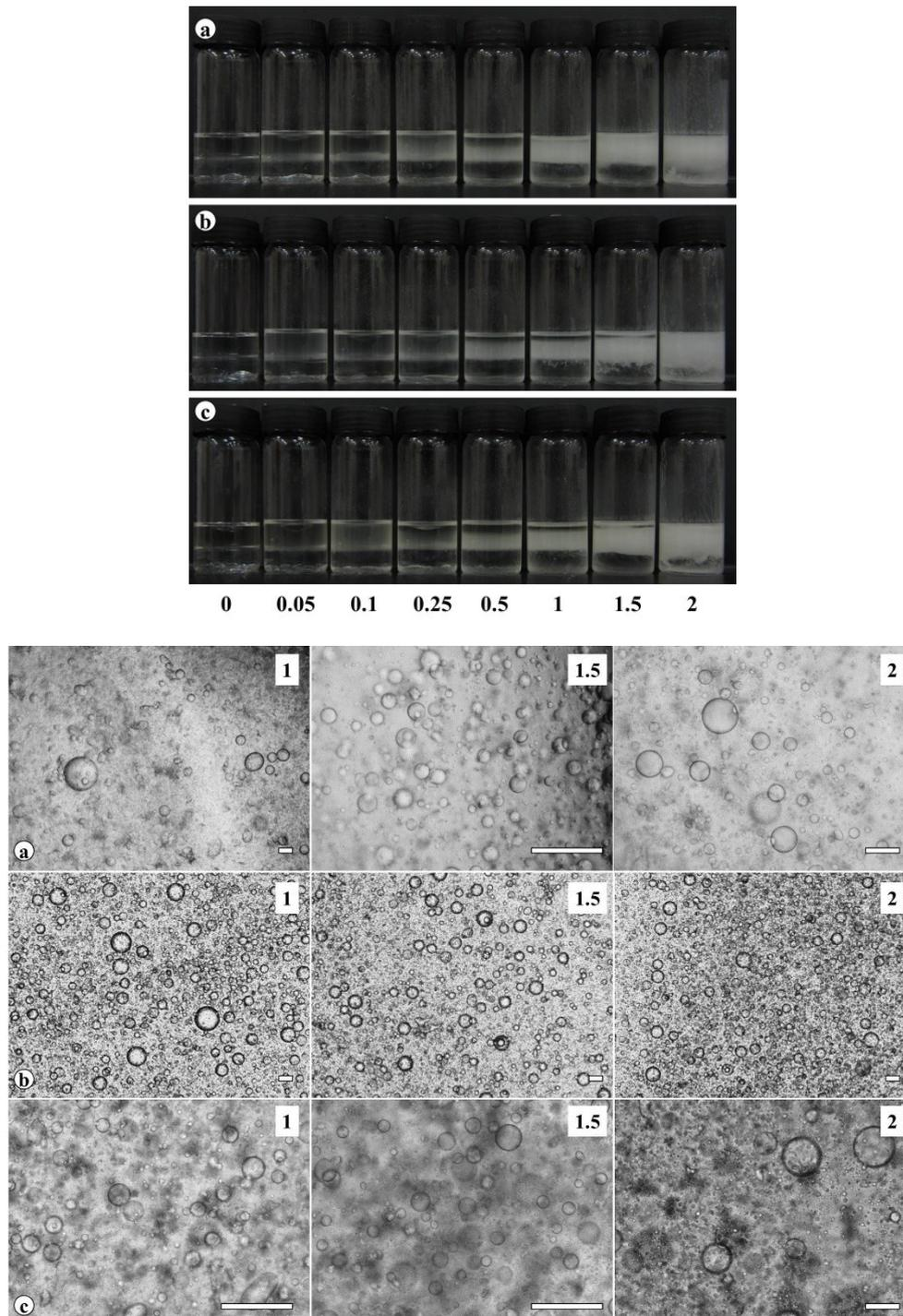
**Figure S7.** (upper) Photographs of glass vials containing olive oil-in-PDMS (a) 20 cS and (b) 50 cS emulsions (1:1, 1 month after preparation) stabilised by different concentrations (given, wt.%) of PF-5 Eight Pearl 300S-A1 sericite particles. (lower) Corresponding optical micrographs of the emulsions stabilised by the given concentrations (wt.%) of particles. The average droplet diameter of the emulsions is also given.
