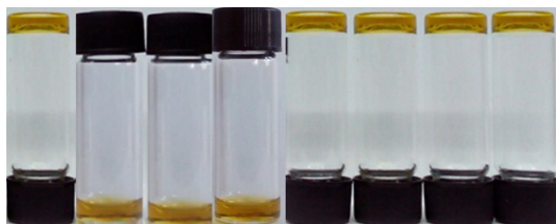
Figure S4. Photographs of the 3 (-Phe-Phe-) gel (toluene, 6 mg/mL) upon the addition of 3.0 equiv. of each anion. From left to right: native gel, + F - , Cl - , H 2 PO 4 - , Br - , I - , HSO 4 - , AcO - .
