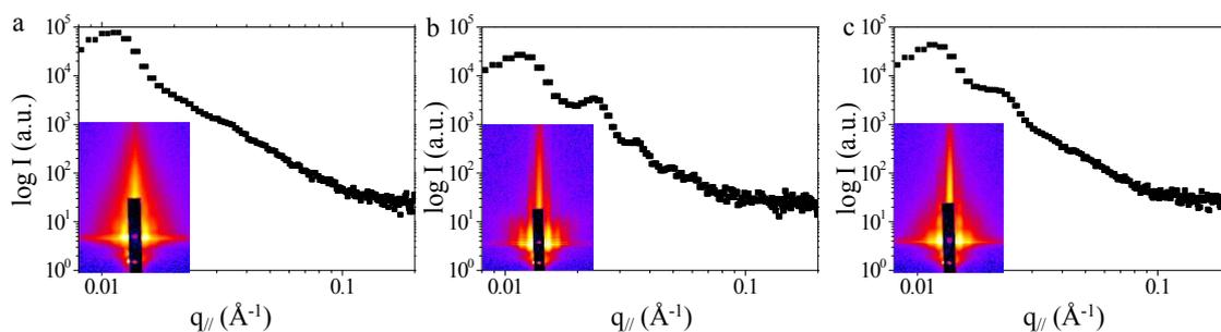
Figure S5 GISAXS 1D profiles of lamellar nanodomains of PS-*b*-PMMA on a PS film having different contact angle values: (a) 90.7°, (b) 79 ° and (c) 70.4 °. Inserts show the corresponding 2D patterns.
