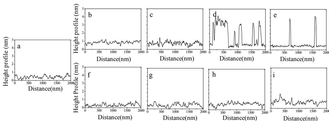
Figure S1 Cross-sectional height profiles of the AFM topographic images of PS films before (a) and after UVIA (b-e) or UVIN (f-i) of varied extent: (b&f) 10, (c&g) 60, (d&h) 360, and (e&i) 540 min.
