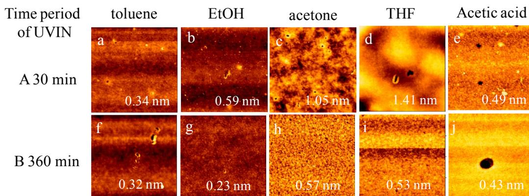
Figure S3 2×2 μm<sup>2</sup> AFM topographic images of the surface of the PS-covered SiO<sub>x</sub>/Si substrate after UVIN treatment of varied extent, (A) 30, and (B) 360 min, followed by immersion in organic solvents: toluene, ethanol, acetone, THF and acetic acid. Mean surface roughness values measured by AFM are designated in the images.
