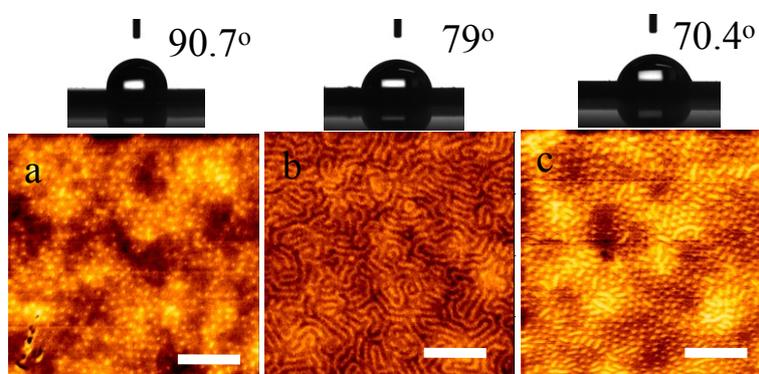
Figure S4 AFM topographic images of lamellar nanodomains of PS-*b*-PMMA on a PS film having different contact angle values: (a) 90.7°, (b) 79° and (c) 70.4°. Scale bar: 500 nm.
