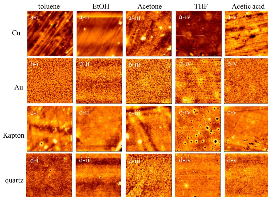
Figure S7  $2 \times 2 \mu\text{m}^2$  AFM topographic images of the surface of the PS-covered substrates of four types (such as (a) Cu, (b) Au, (c) kapton and (d) quartz) after UVIN of 6 h, followed by immersion in organic solvents: (i) toluene, (ii) ethanol, (iii) acetone, (iv) THF and (v) acetic acid.
