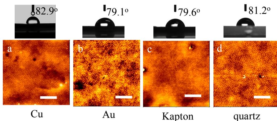
Figure S8 AFM topographic images of PS-*b*-PMMA films on a PS layer of initial thickness 7.7 nm and with a neutral surface property over (a) Cu, (b) Au, (c) Kapton, and (d) quartz. Scale bars: 500 nm.
