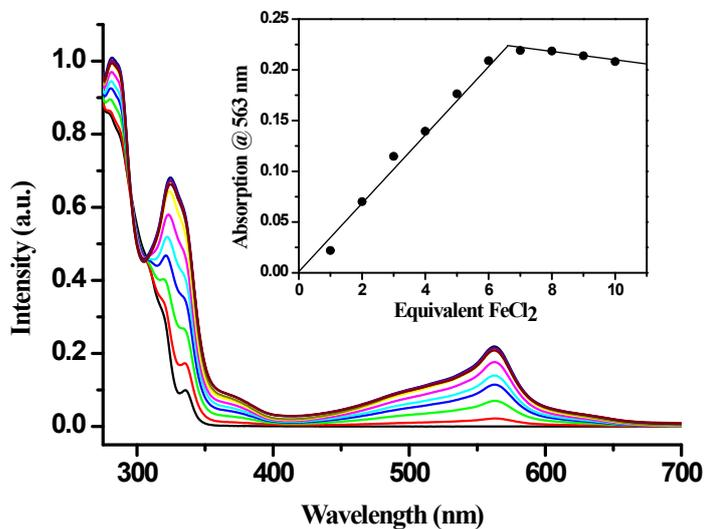
**Figure S3.** UV-vis spectra of S'-Tpy chloroform solution titrated with FeCl<sub>2</sub> methanol solution. Inset is the plot of the absorbance at 325 nm *versus* the equivalents of FeCl<sub>2</sub>.
