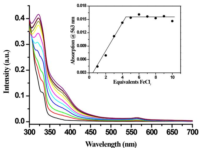
**Figure S4.** UV-vis spectra of SI-Tpy chloroform solution titrated with FeCl<sub>2</sub> methanol solution. Inset is the plot of the absorbance at 325 nm *versus* the equivalents of FeCl<sub>2</sub>.
