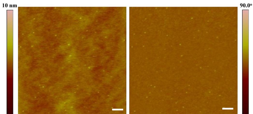
**Figure S5.** AFM height image (the left) and phase image (the right) of SI-Tpy diblock copolymer. The scalar bar represents 100 nm.
