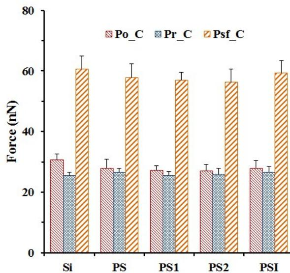
**Figure S5.** Adhesion forces for three clean pollen particles of each species (Po\_C, Pr\_C and Psf\_C) interacting with five different substrate surfaces (Si, PS, PS1, PS2 and PSI) under load force 2.5 nN. Error bars are 95% confidence intervals.
