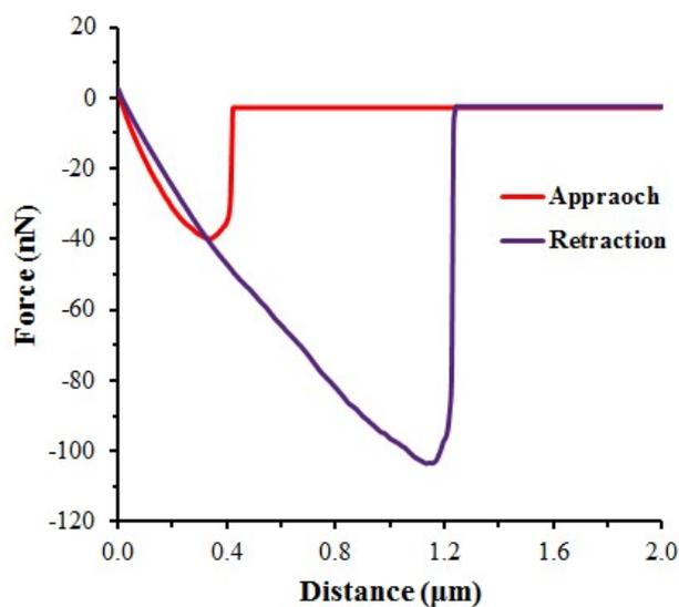
**Figure S3.** A typical force-distance curves for the interactions of a clean sunflower pollen AFM probe (Psf\_C, spring constant 0.5 N/m) and a flat PDMS substrate at 2.5 nN load forces: the gradient in the contact region was  $0.08 \pm 0.01$  N/m.
