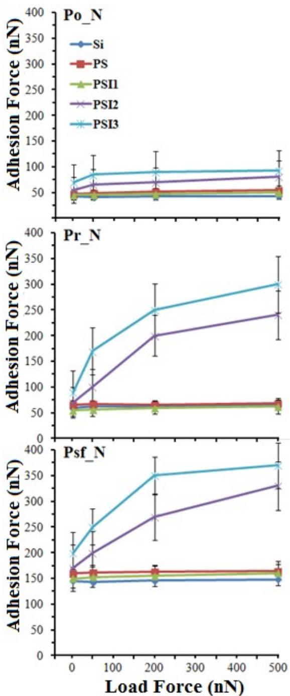
**Figure S7.** Adhesion forces versus load forces for the native pollen particles interacting with five different substrate surfaces. Error bars are 95% confidence intervals.
