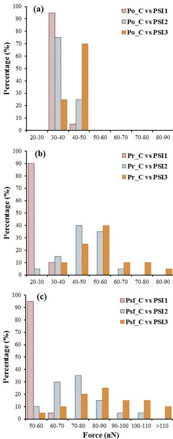
**Figure S4.** Force-distributions for the interactions of pollen AFM probes (a: Po\_C; b: Pr\_C; c: Psf\_C) with three PSI-PS substrates under 2.5 nN load force.
