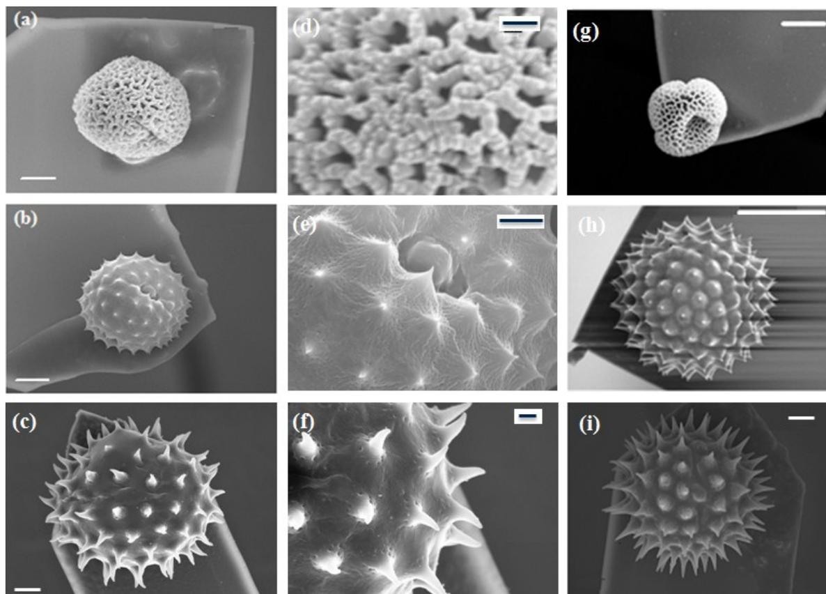
**Figure S1.** SEM images of AFM colloidal-probes of the pollen grains glued to the end of tipless AFM cantilevers. (a) and (d) are the native olive pollen particles; (b) and (e) are the native ragweed pollen particles; (c) and (f) are the native sunflower pollen particles; (g), (h), and (i) the clean particles of olive, ragweed and sunflower pollens respectively. The white scale bar represents 10  $\mu\text{m}$  and the black scale bar is 1  $\mu\text{m}$ .
