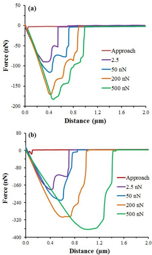
**Figure S6.** Force-distance curves for the interactions of sunflower pollen AFM probes (a: Psf\_C; b: Psf\_N) and PSI3 substrate at a series of load forces.
