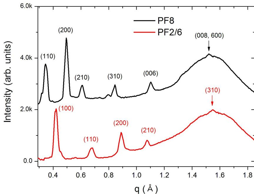
**Figure S1.** X-ray diffraction patterns of annealed PF8 (upper plot, black) and PF2/6 (lower plot, red) after rubbing of the film surfaces. Direction of scattering vector was changed during the detector scanning. Edge to edge interlayer spacing is  $\sim 16.5 \text{ \AA}$  and  $\sim 16 \text{ \AA}$  for PF8 and PF2/6, respectively. Peak (006) and (008) indicates the polymer chain orientation of PF8.<sup>1-6</sup>
