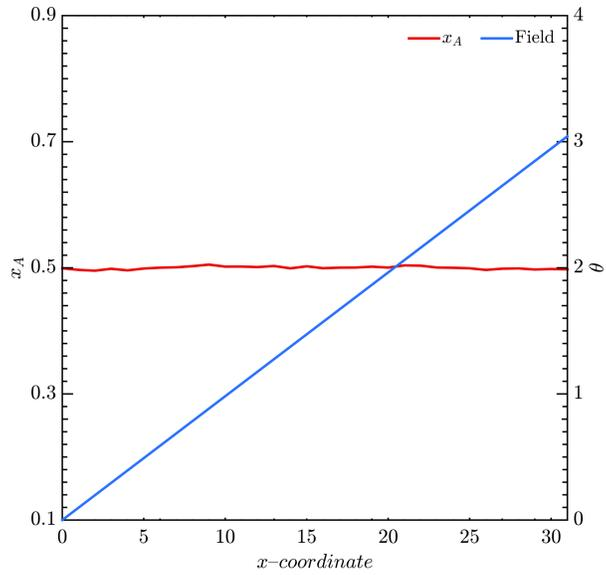
Figure 1. The application of a linear field to the binary mixture  $\varepsilon_{AA}/\varepsilon_{BB} = T^* = 0.40$ , with  $x_B = 0.5$ . No segregation is observed in the system, highlighting the role of nonlinear stress in inducing elastically-driven demixing.
