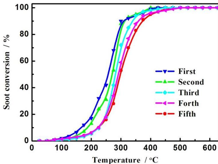
**Figure S5.** The reusability of the sample CuMn-HBeta in the soot catalytic oxidation (Reaction condition: 10% O<sub>2</sub>; 500 ppm NO in N<sub>2</sub>; total flow is 200 mLmin<sup>-1</sup>; the space velocity is 120000 h<sup>-1</sup>; W/F = 0.03 (g·s)/mL; the mass ratio (catalyst/soot) is 10:1).
