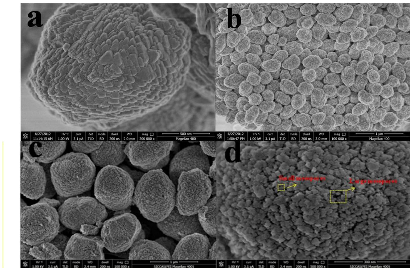
**Figure S1.** FE-SEM images of the samples a) Beta, b) MBeta and c-d) HBeta at low and high-magnifications.
