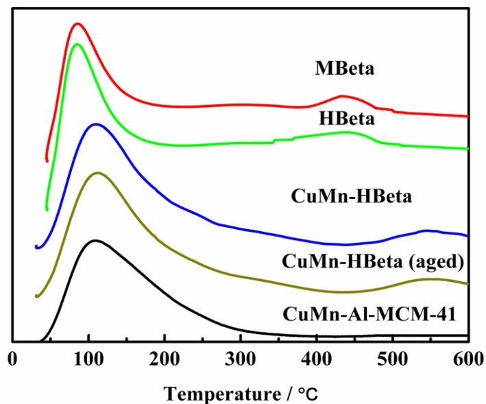
**Figure S4.** NH<sub>3</sub>-TPD profiles of CuMn-HBeta and the reference CuMn-Al-MCM-41 with a similar pore size of 7-50 nm.
