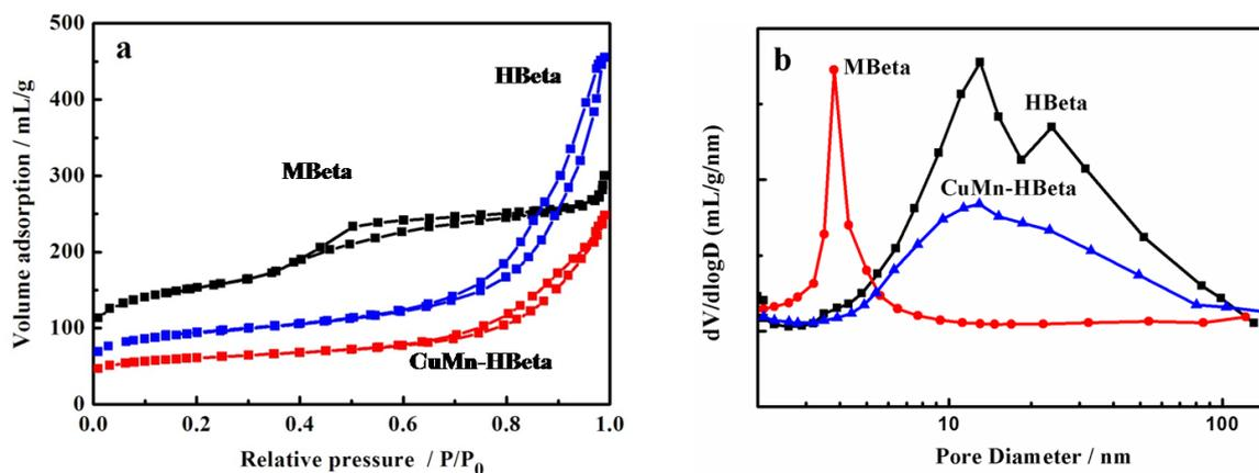
**Figure S3.** a) N<sub>2</sub> adsorption/desorption isotherms and b) the corresponding pore size distributions of the samples MBeta, HBeta and CuMn-HBeta.
