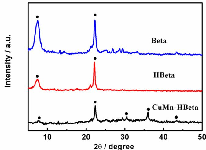
**Figure S2.** XRD profiles of the samples Beta, HBeta and CuMn-HBeta (●: zeolite Beta; ◆Cu<sub>1.5</sub>Mn<sub>1.5</sub>O<sub>4</sub>).
