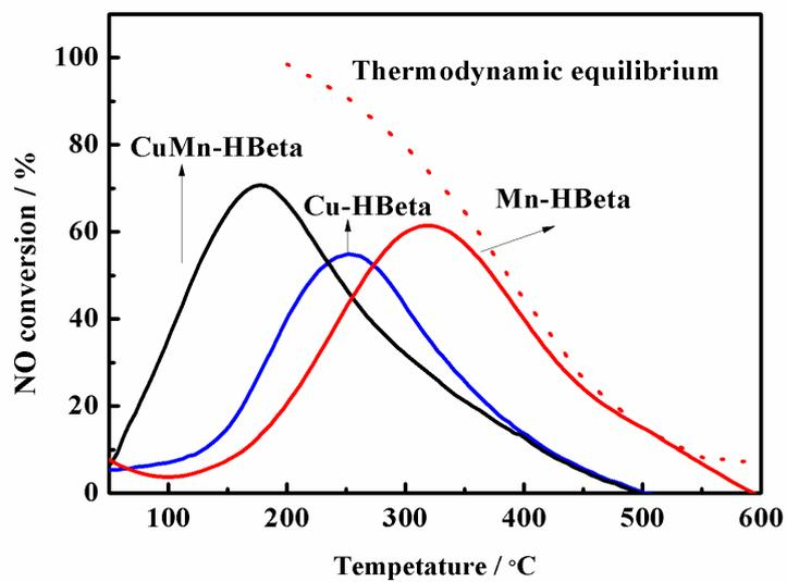
**Figure S8.** The oxidation activity of NO to NO<sub>2</sub> by O<sub>2</sub> over the sample CuMn-HBeta and the references Cu-HBeta and Mn-HBeta.
