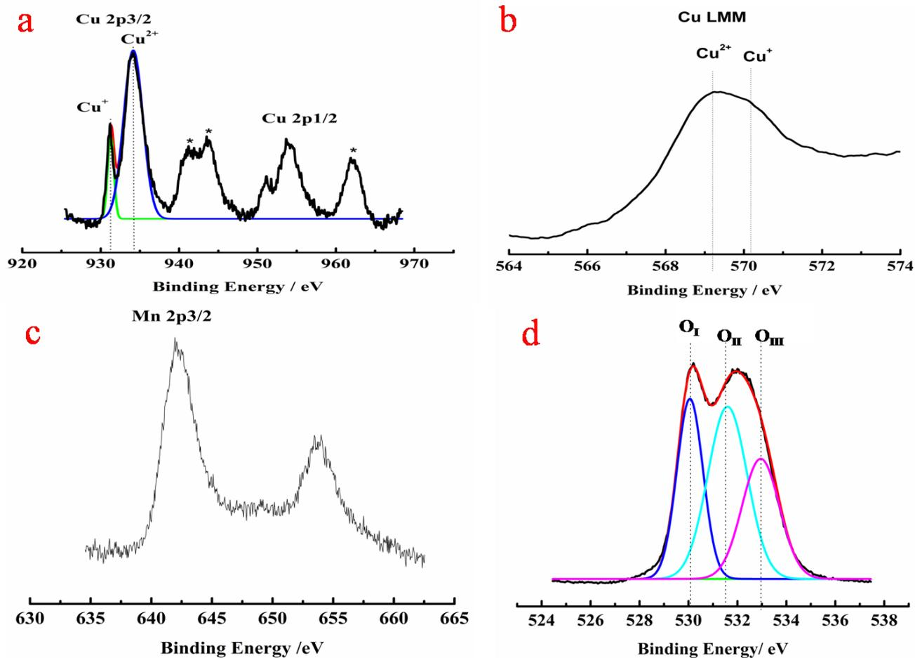
**Figure S7.** a) Cu 2p photoelectron spectrum, b) Cu LMM Auger spectrum, c) Mn 2p and d) O 1s photoelectron spectra of CuMn-HBeta. Peak fitting is carried out on the 2p 3/2 peak of Cu and Mn element.
