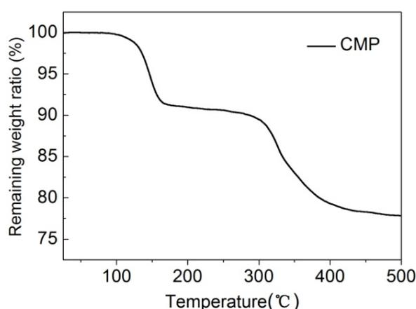
**Fig. S1** Thermogravimetric (TG) curve of  $(\text{C}_2\text{N}_2\text{H}_{10})\text{Mn}_2(\text{PO}_4)_2 \cdot 2\text{H}_2\text{O}$  nanosheets
