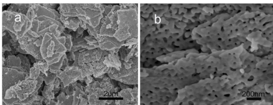
**Fig. S2** Supplementary SEM images of  $\text{LiMnPO}_4$ : (a) low resolution, and (b) high resolution.
