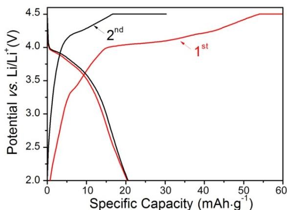
**Fig. S4** Charge-discharge curves of pure LiMnPO<sub>4</sub> at 0.1C.
