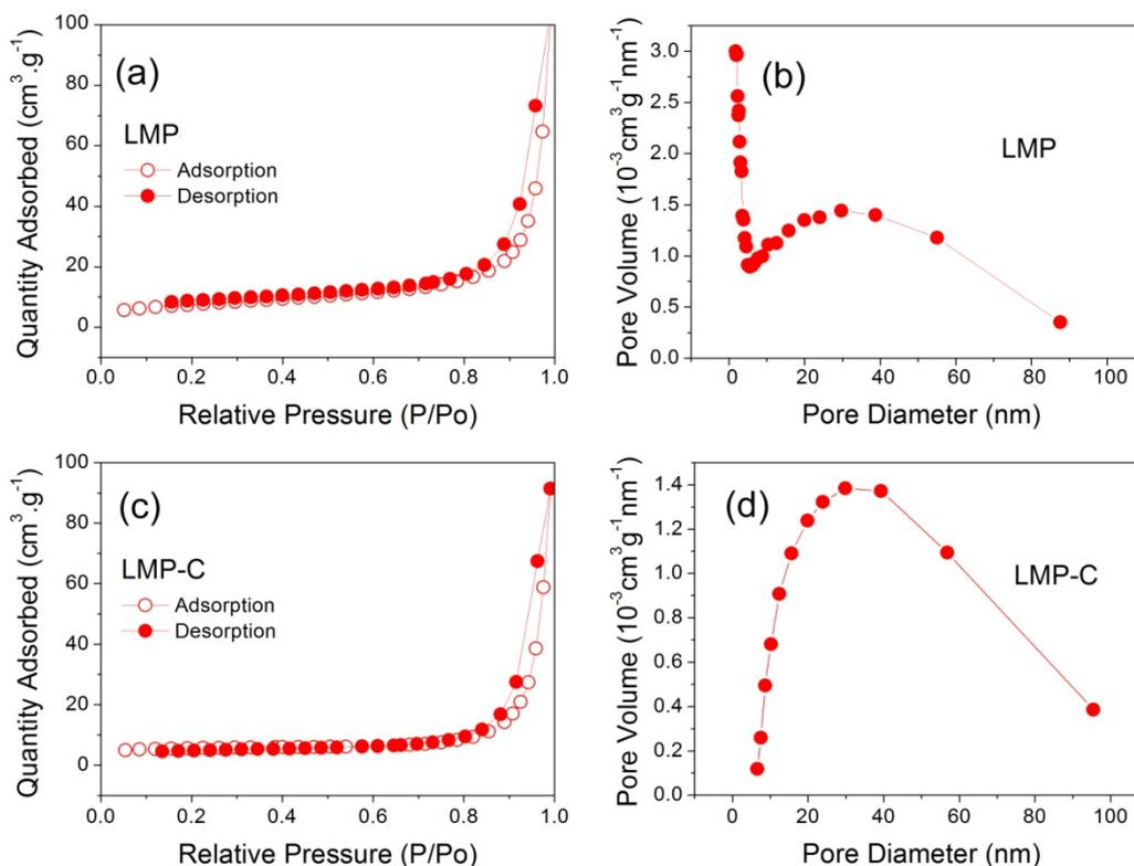
**Fig. S3** Nitrogen adsorption and desorption isotherm (a, c) and BJH adsorption pore size distribution (b, d) of porous nanoflake structured  $\text{LiMnPO}_4$  (LMP) and  $\text{LiMnPO}_4\text{-C}$  (LMP-C), respectively.
