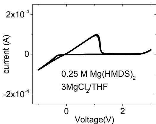
Figure S3. Cyclic Voltammetry of 0.25 M  $\text{Mg}(\text{HMDS})_2\text{-}3\text{MgCl}_2$  in THF. The working electrode is Pt electrode, and Mg ribbon is used both as the reference and the counter electrode. The scan rate is  $100 \text{ mV s}^{-1}$  and the number of cycles is marked on the graph.
