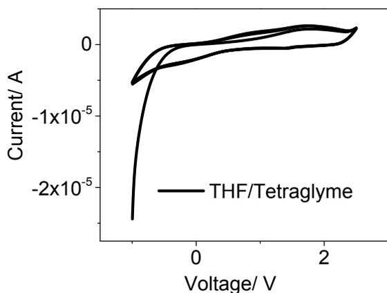
Figure S2. Cyclic Voltammetry of 0.5 M  $\text{Mg}(\text{HMDS})_2\text{-}4\text{MgCl}_2$  in THF/DME (1:1), THF/Diglyme (1:1), THF/triglyme (1:1), THF/tetraglyme (1:1). The working electrode is Pt electrode, and Mg ribbon is used both as the reference and the counter electrode. The scan rate is  $100 \text{ mV s}^{-1}$  and the number of cycles is marked on the graph.
