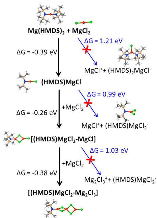
**Figure S1.** Main reaction pathway (in black arrow) and other less possible reactions we calculated. Reaction free energies (corresponding to 1 mole of each reactant) of these steps are reported.
