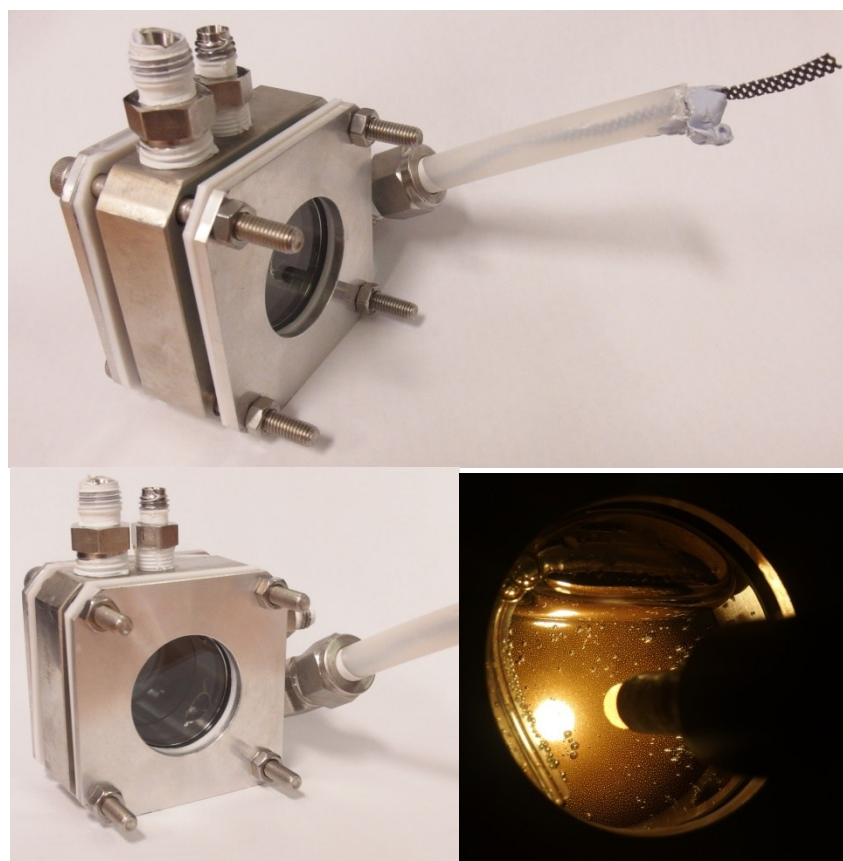
Fig. S1: New cell setup in metal cell with separated counter electrode compartment, direct access to headspace and improved sealing. Area of the film is determined to be 6.79 \text{ cm}^2
