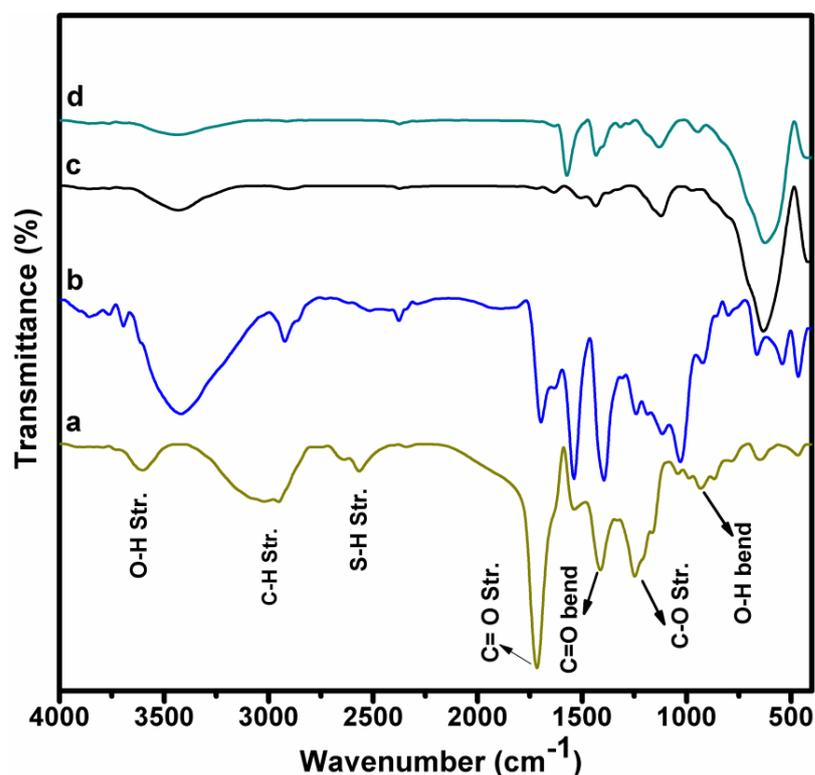
**Fig. S1** FTIR spectra of (a) Mercaptopropionic acid (b) R-CdSe QDs (c) STO and (d) R-CdSe-MPA-STO photo electrodes.
