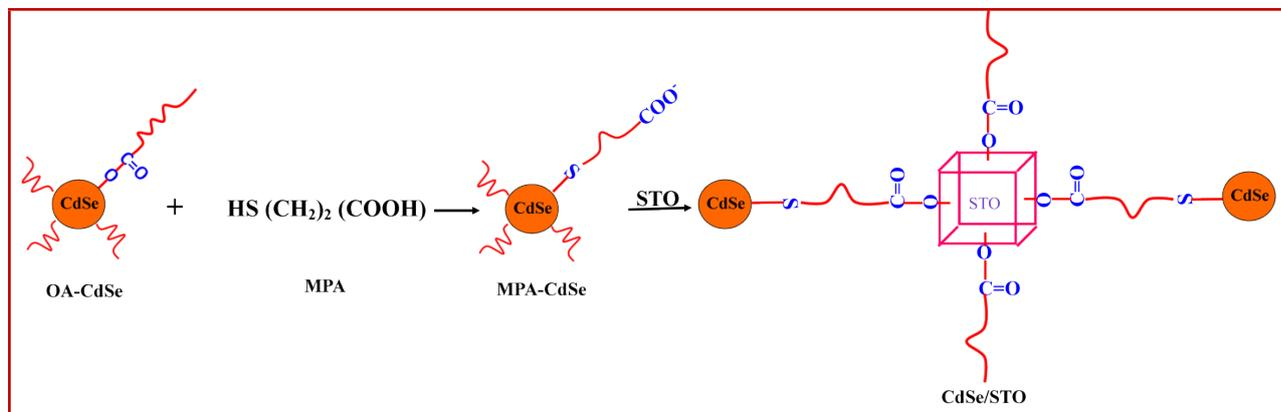
**Scheme S-I.** Schematic representation of CdSe QDs sensitization on STO nanocubes.
