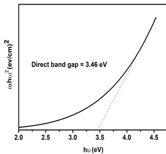
**Fig. S3** Tauc Plot for STO photo electrode.
