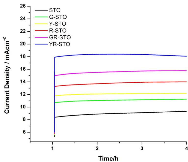
**Fig. S4** i-t curves of STO and CdSe sensitized STO photo electrode under illumination condition.
