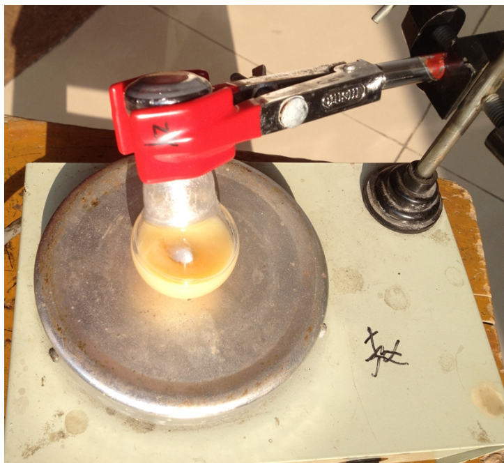
Fig. S2 The photo of outdoor equipment of sunlight-driven water splitting by \text{g-C}_3\text{N}_4/\text{MoS}_2 -2.89% system in Wuxi city on Nov. 18 2014. Outdoor temperature: 9-14 °C, Time: 09:00-15:00.
