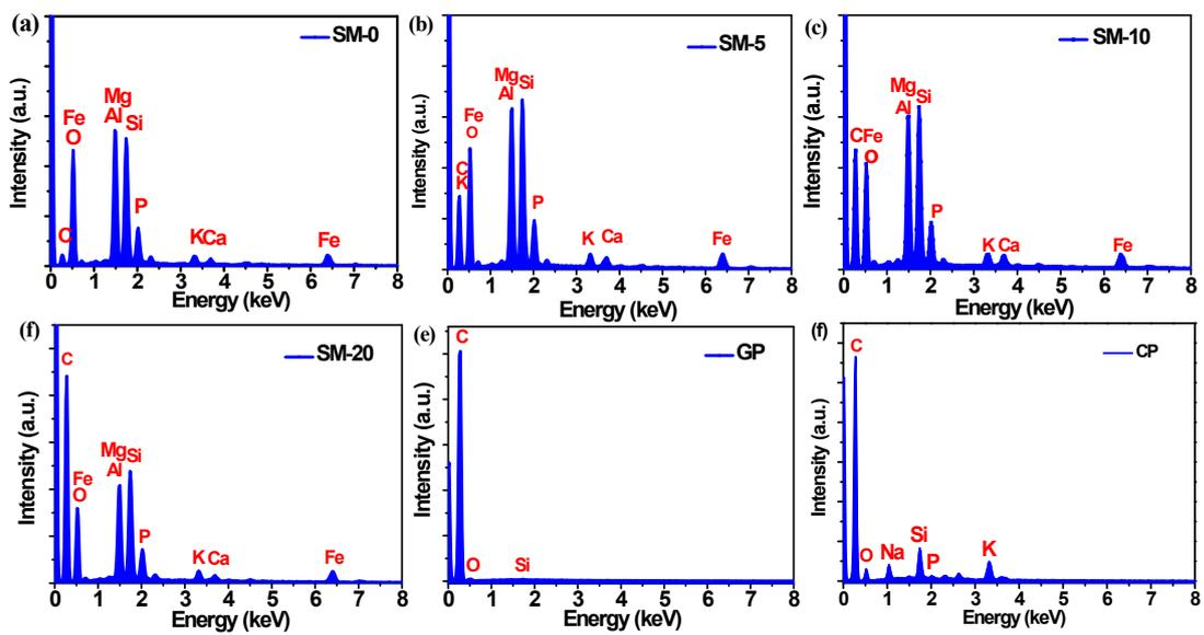
Figure S2. EDX spectrum showing the elemental composition of the resultant anodes.
