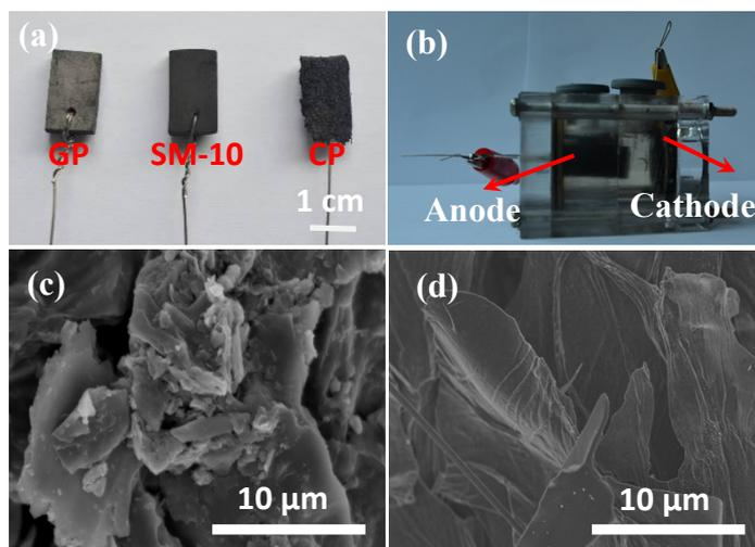
**Figure S1.** (a) Photographic illumination of the as-prepared anodes; (b) photographic image of the MFC equipped with the as-prepared anodes; (c) SEM image of the graphite plate (GP) anode; (d) SEM image of the coconut shell-derived carbon plate (CP) anode.
