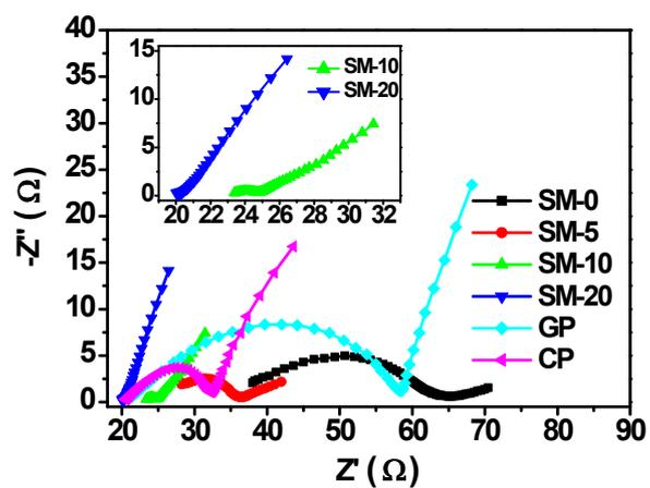
**Figure S6. (a)** Nyquist plots of the different anodes in the MFCs after inoculation. The inset contains Nyquist plots of the SM-10 and SM-20 anodes.
