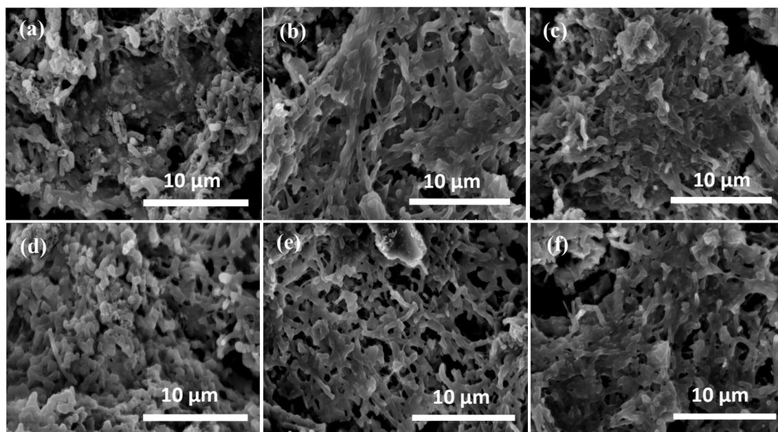
**Figure S5.** SEM images of the electroactive biofilm grown on the (a) SM-0, (b) SM-5, (c) SM-10, (d) SM-20, (e) GP and (f) CP andoes.
