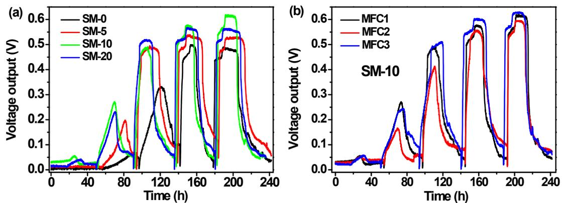
**Figure S4.** (a) Voltage output versus time curves during start-up of the MFCs with various anodes with a 1 k $\Omega$  resistance loading; (b) Voltage output versus time curves of three parallel MFCs with the SM-10 anode.
