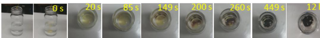
**Fig. S3.** Sequence of photographs after adding drops of MAPbI<sub>3</sub> precursor solution (in NMP) in DEE bath showing sluggish MAPbI<sub>3</sub> perovskite precipitate formation.
