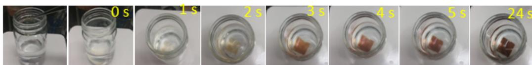
**Fig. S2.** Sequence of photographs after dropping a spin-coated MAPbI<sub>3</sub> precursor thin film (patterned) in DEE bath showing rapid MAPbI<sub>3</sub> perovskite thin film formation.
