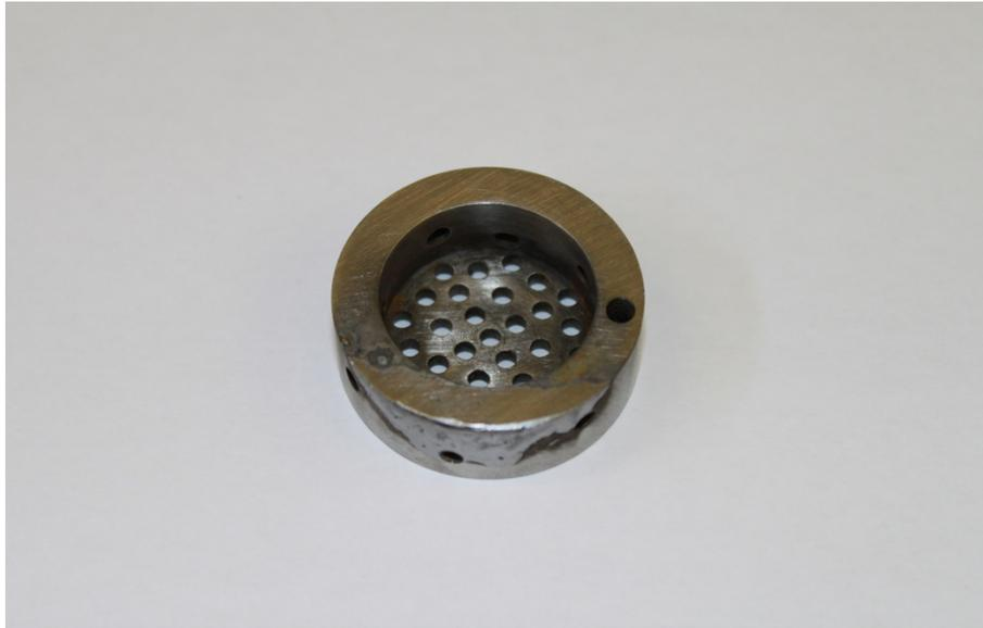
Figure S2: The stainless steel cup used as a cathode current collector. The cathode was connected to the power supply *via* stainless steel rod connected on the sidewall of the cup.
