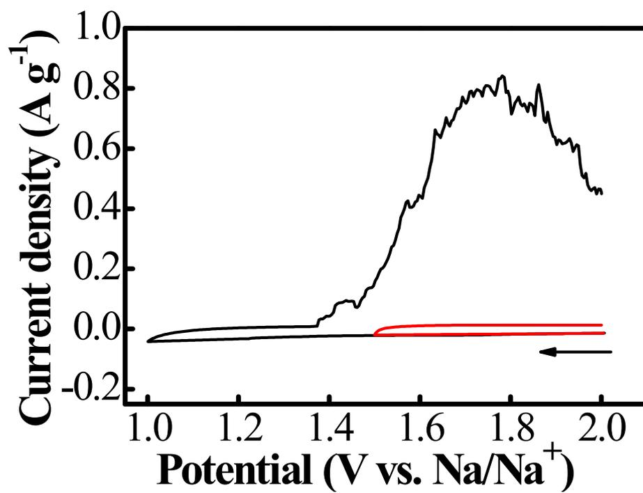
Fig. S3 CV curves of AC electrode with potential limits of 1.0 and 1.5 V. Potential was scanned from 2 V with a rate of 0.1 mV s<sup>-1</sup>.
