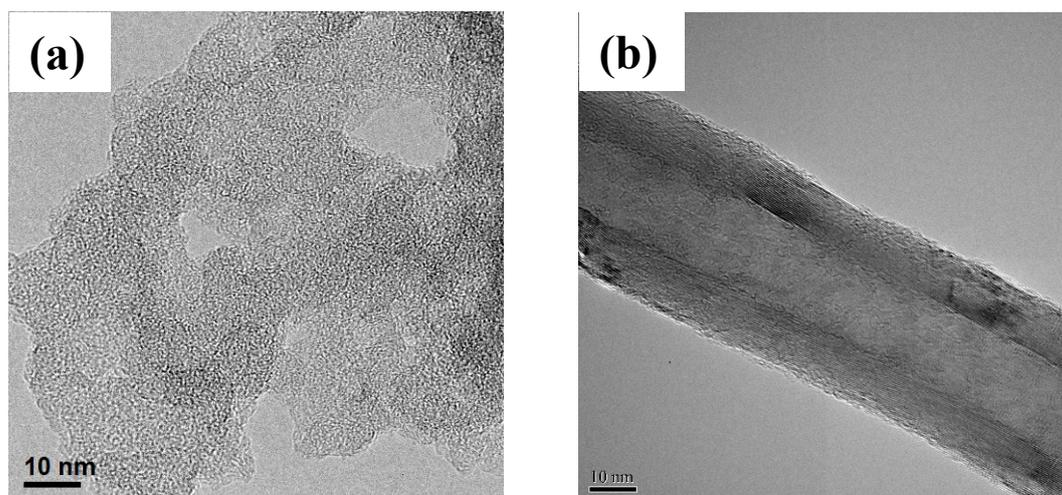
Fig. S1 TEM micrographs of (a) CNT and (b) AC.
