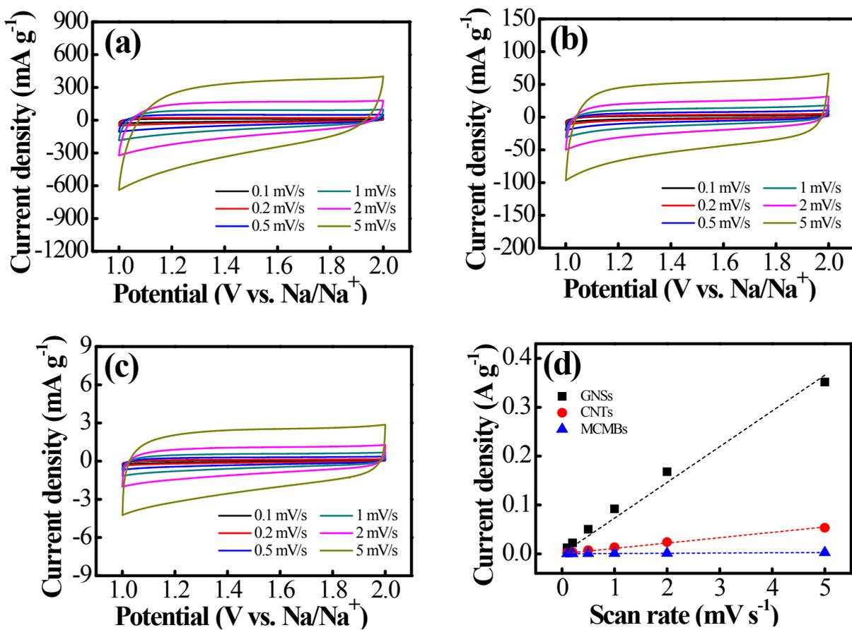
Fig. S2 CV curves of (a) GNS, (b) CNT, and (c) MCMB electrodes recorded in potential range of 1.0–2.0 V with various scan rates. (d) CV response current as function of potential scan rate for GNS, CNT, and MCMB electrodes.
