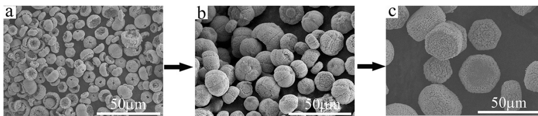
Figure S1. The morphology evolution of Zn-Fe-ZIF, (a) hollow hemisphere (the molar ratio of \text{Zn}^{2+} to \text{Fe}^{2+} = 3), (b) pumpkin (the molar ratio of \text{Zn}^{2+} to \text{Fe}^{2+} = 4), (c) hexagonal prisms (the molar ratio of \text{Zn}^{2+} to \text{Fe}^{2+} = 5).
