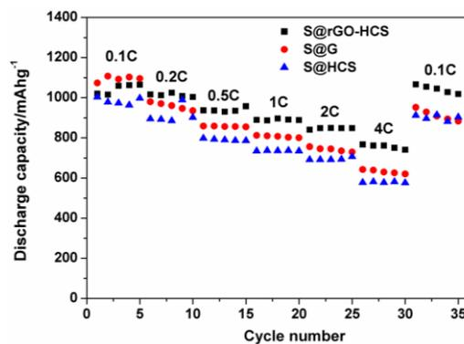
**Figure S6** Rate performance of the S@rGO-HCS, S@HCS, and S@G electrode
