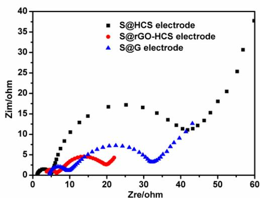
**Figure S8** Nyquist plots for the S@rGO-HCS, S@HCS and S@G electrodes in the frequency range of 100 mHz to 100 kHz
