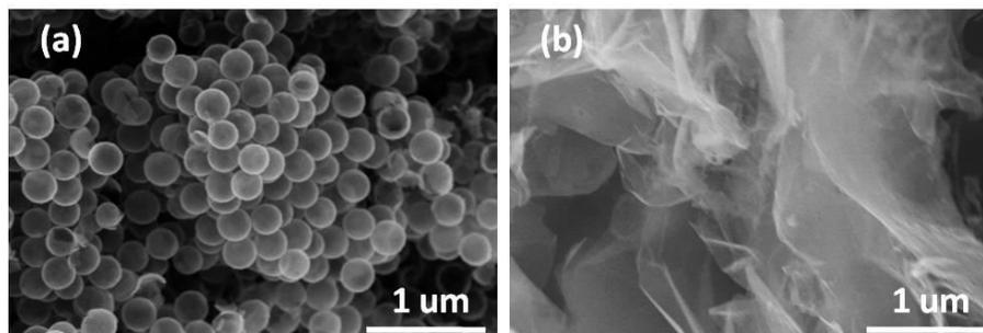
**Figure S5** SEM images of (a) S@HCS and (b) S@G nanocomposite
