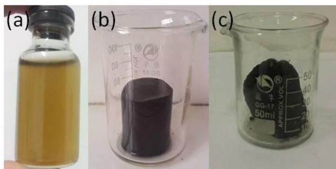
**Figure S1** optical photographs of the (a) GO solution, (b) 3D GO-RF@SiO<sub>2</sub> wet gel, and (c) rGO-RF@SiO<sub>2</sub> gel
