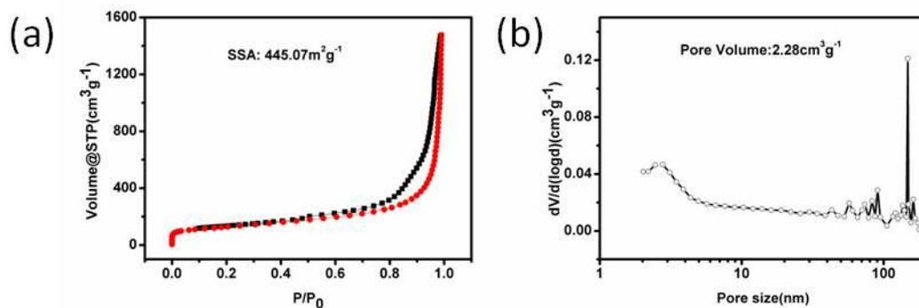
**Figure S3** N<sub>2</sub> adsorption isotherms and pore-size distribution of 3D rGO-HCS nanocomposite.
