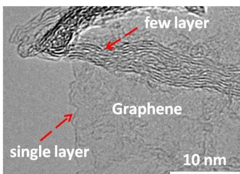
**Figure S2** selected high resolution TEM image of the 3D rGO-HCS nanocomposite.
