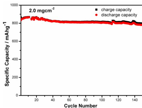
**Figure S8** Cycling performance of the S@rGO-HCS electrode with sulfur mass loading of  $2.0 \text{ mg cm}^{-2}$  at 0.5C rate
