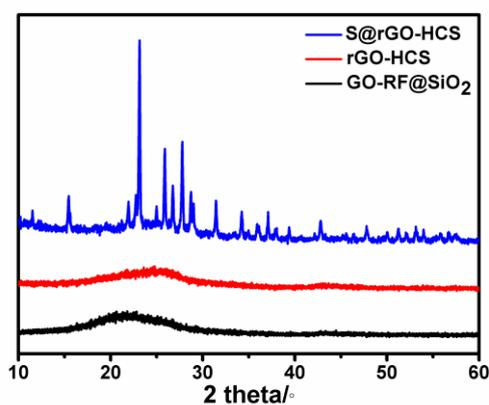
**Figure S4** XRD patterns of 3D GO-RF@SiO<sub>2</sub>, 3D rGO-HCS and the S@rGO-HCS nanocomposite
