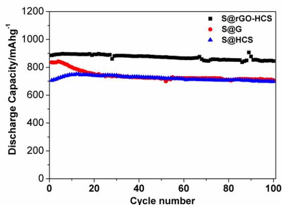
**Figure S7** Cycling performance of the S@rGO-HCS, S@HCS, and S@G electrode at 1C rate
