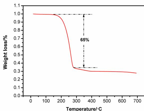
**Figure S9** Thermogravimetric analysis of the S@rGO-HCS nanocomposite, which were carried out at a flow rate of 10 °C/min under N<sub>2</sub> flow
