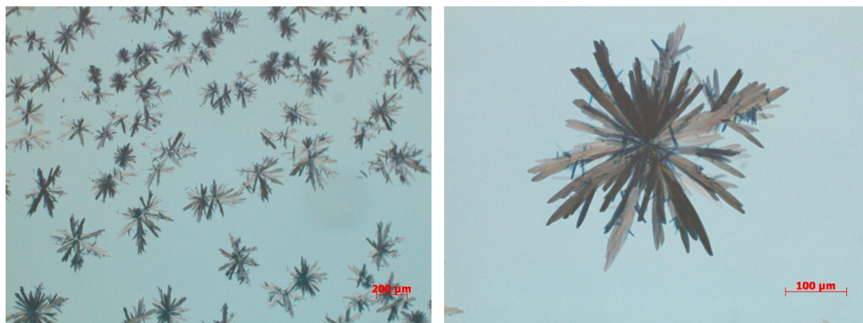
Figure S14: Microscope images of a saturated p-DTS(FBTTh2)2 solution near 30degC. Images taken at 5x (left) and 20x (right) magnification.
