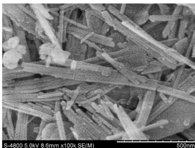
Fig. S2 A typical SEM image of attapulgite.
