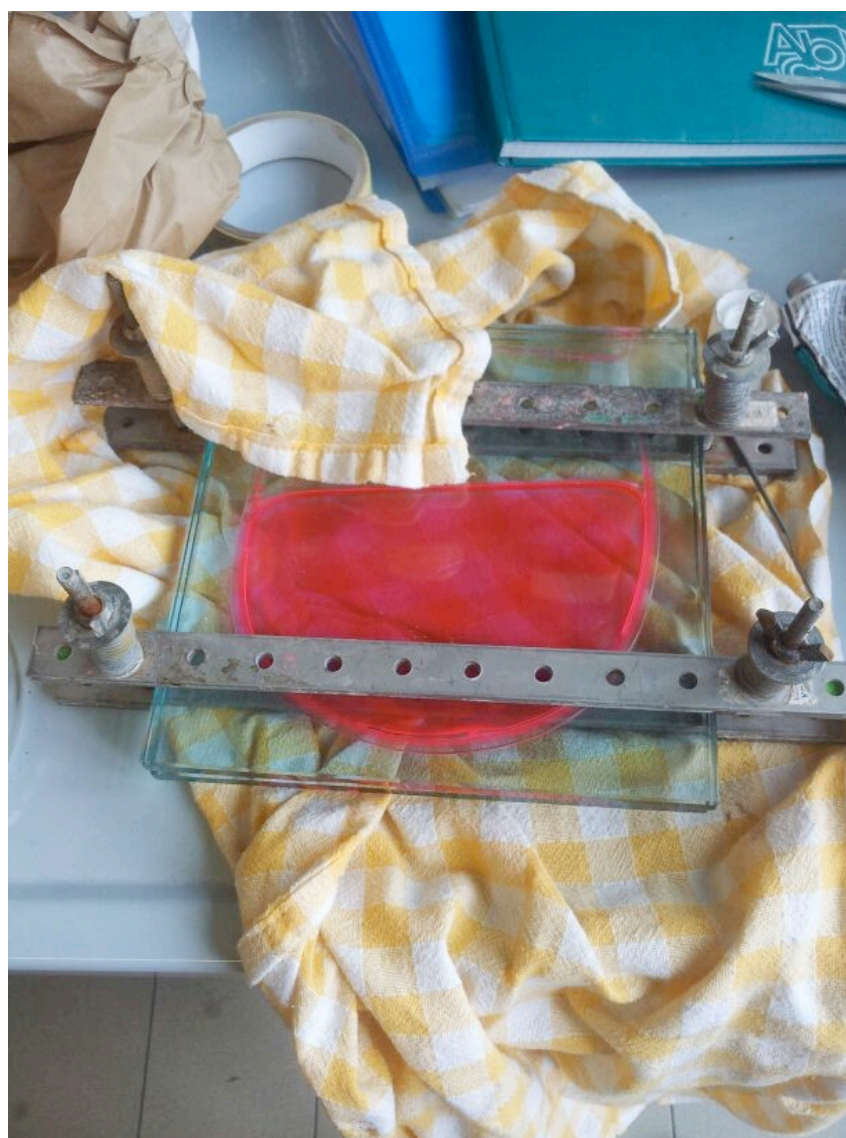
Figure S9. Experimental setup for the cell cating of the PMMA based LSC.
