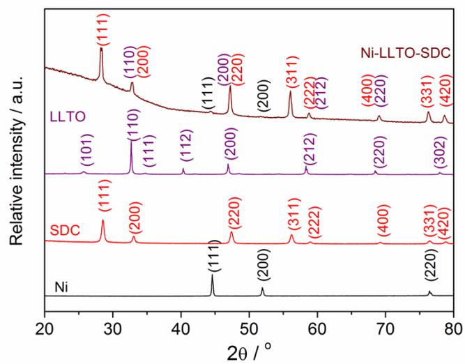
**Figure S4** XRD patterns of Ni-LLTO co-infiltrated SDC anodes after calcination at 900 °C for 2 hours, as well as the pure phases such as Ni, SDC and LLTO.
