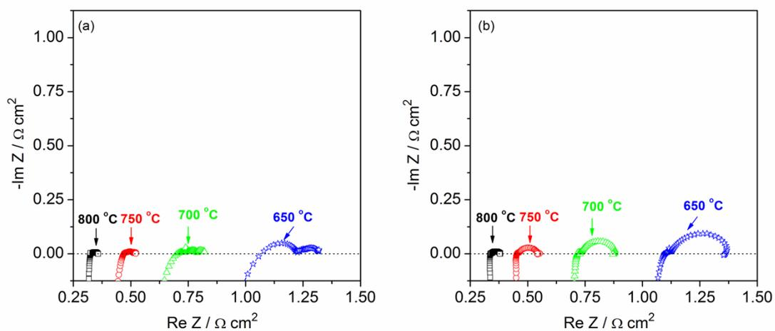
**Figure S6** EIS spectra of the fuel cell with Ni-LLTO co-infiltrated SDC anode operating on  $\text{H}_2$  (a) and 1000 ppm  $\text{H}_2\text{S}-\text{H}_2$  (b) fuels at 800 °C.
