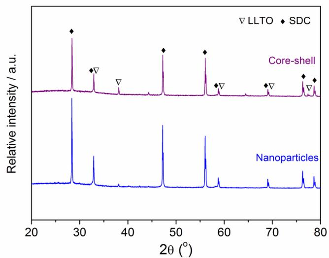
**Figure S2.** XRD patterns of LLTO-infiltrated SDC anodes after long-term operation using 1000 ppm  $\text{H}_2\text{S}$ - $\text{H}_2$  fuel.
