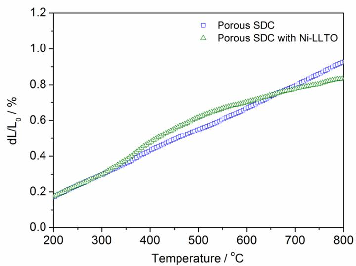
**Figure S5** Thermal expansion behaviors of the porous SDC and Ni-LLTO co-infiltrated SDC bars sintered at 900 °C.
