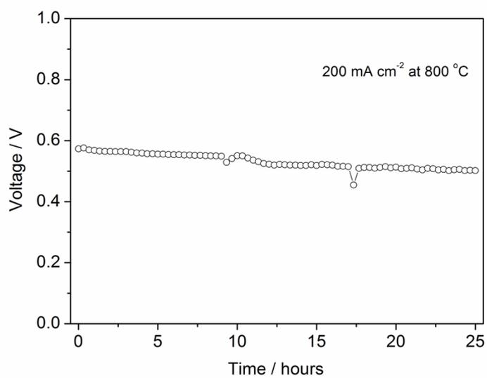
**Figure S7** Time-dependent voltage of the fuel cell with Ni-LLTO co-infiltrated SDC anodes operating on 1000 ppm H<sub>2</sub>S-H<sub>2</sub> under a current density of 200 mA cm<sup>-2</sup> at 800 °C.
