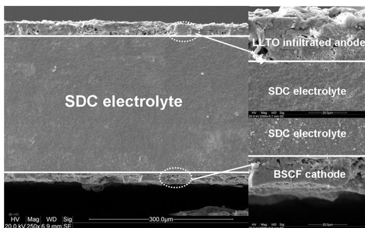
**Figure S1** A typical SEM image of a cross-section of a fuel cell with a LLTO-infiltrated SDC anode.
