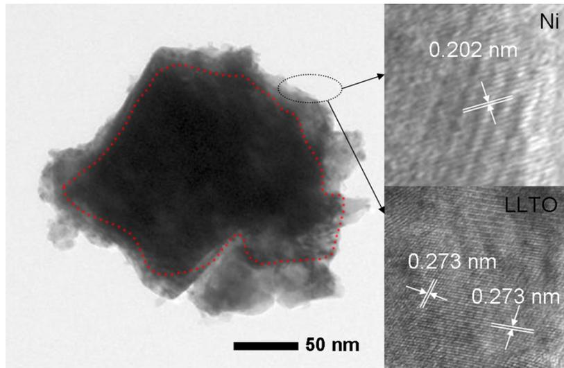
**Figure S3** TEM results under different magnifications of the core-shell structured Ni-LLTO co-infiltrated SDC anodes.
