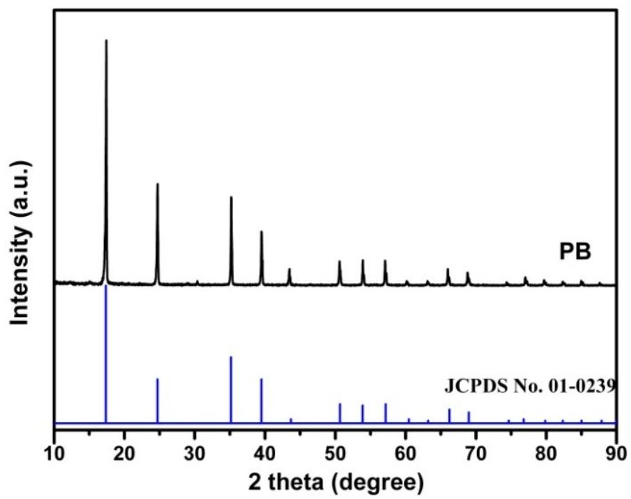
Figure S1 XRD patterns of as-prepared precursor and standard Prussian blue.
