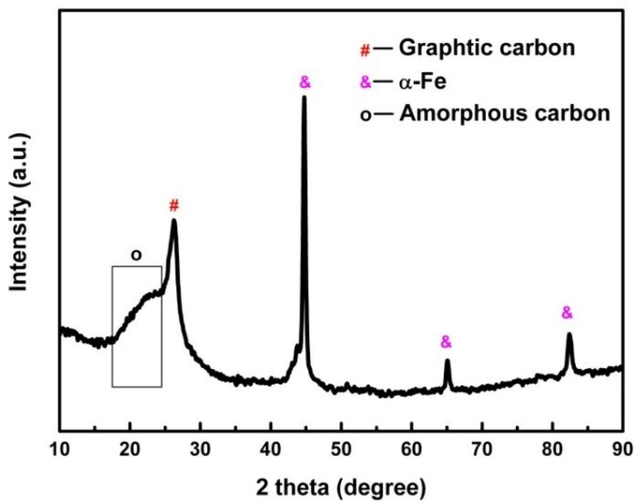
Figure S2 XRD pattern of Fe/C nanocubes after strong acid treatment.
