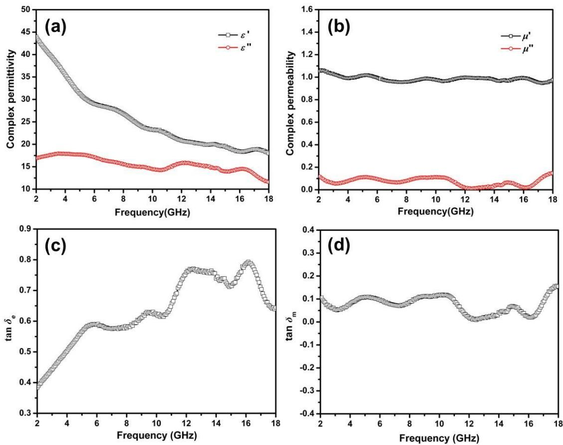
Figure S8 The complex permittivity (a), complex permeability (b), dielectric loss tangent (c) and magnetic loss tangent (d) of S2 after being treated by strong acid.
