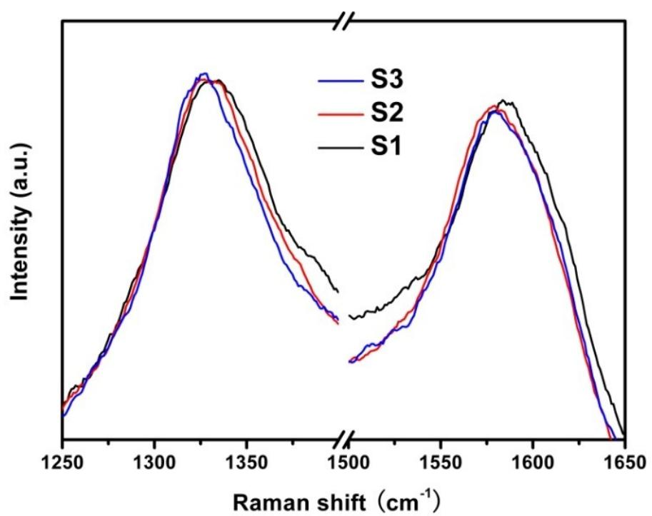
Figure S7 The local enlargements for D- and G-bands in Raman spectra.
