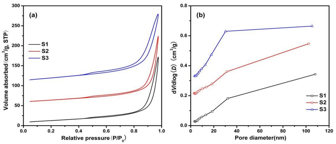
Figure S5  $\text{N}_2$  adsorption-desorption isotherms (a) and pore size distributions (b) of Fe/C composites. The isotherms of S2 and S3 remove upwards 50 and 100  $\text{cm}^3/\text{g}$  at the beginning for clarity, respectively.
