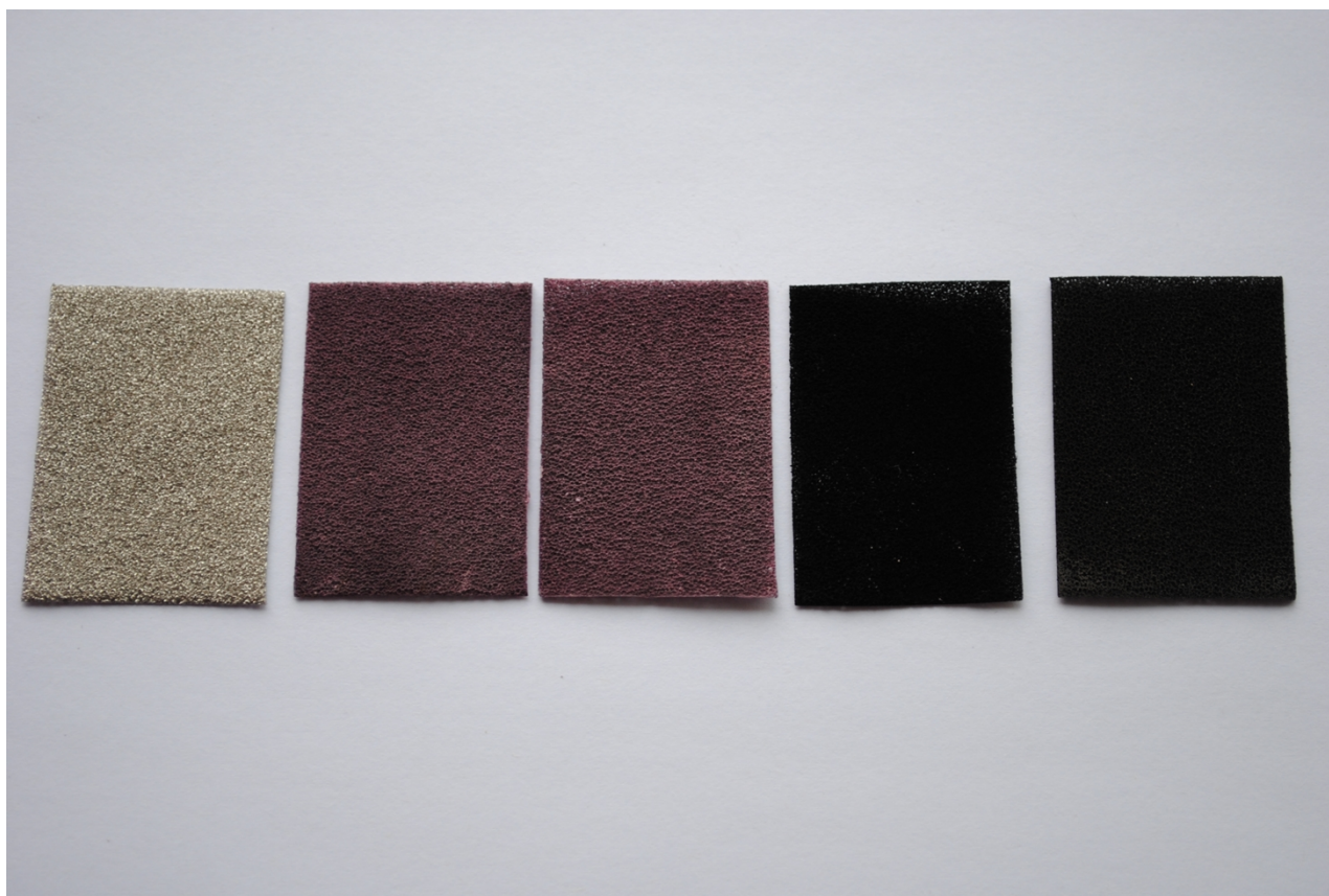
Figure S1 photographs of nickel foam substrate, \text{Co}_3\text{O}_4 precursor on nickel foam, \text{Co}_3\text{O}_4@ \text{CoMoO}_4 precursor on nickel foam, \text{Co}_3\text{O}_4 NWAs on nickel foam and \text{Co}_3\text{O}_4@ \text{CoMoO}_4 NWAs on nickel foam.
