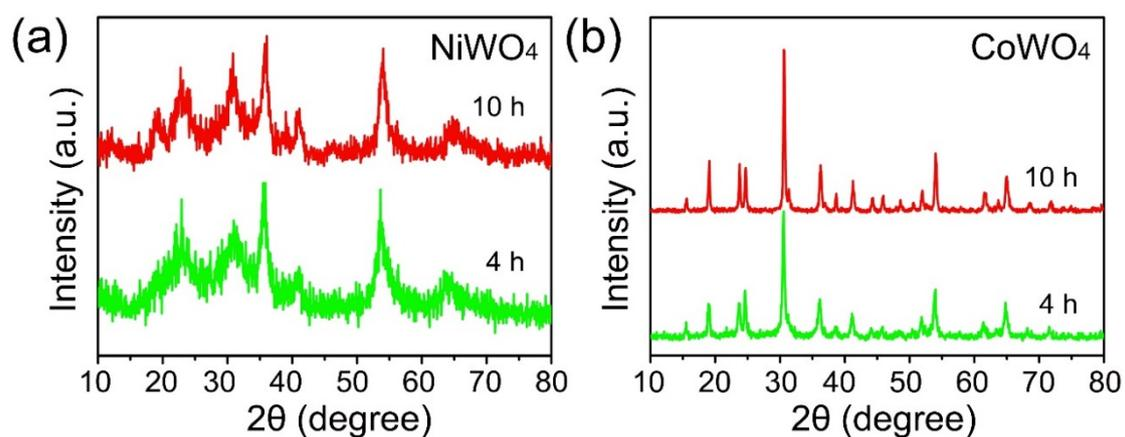
**Figure S1** (a), (b) XRD patterns of NiWO<sub>4</sub>, CoWO<sub>4</sub> samples with different reaction times (green line: 4 h; red line: 10 h).
