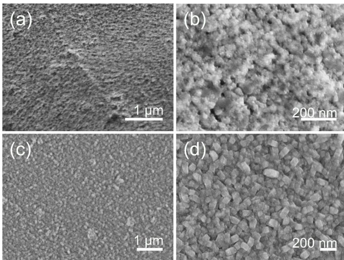
**Figure S8** (a), (b) Low- and high-magnification SEM image of NiWO<sub>4</sub>/Ni foam nanostructures after 6000 cycles at 50 mV s<sup>-1</sup>, respectively; (c), (d) Low- and high-magnification SEM image of CoWO<sub>4</sub>/Ni foam nanostructures after 6000 cycles at 50 mV s<sup>-1</sup>, respectively.
