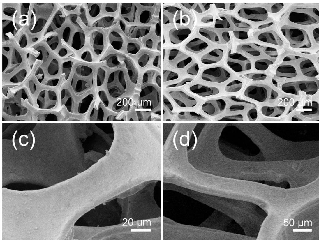
**Figure S3** (a), (b) Lower-magnification SEM image of NiWO<sub>4</sub>/Ni foam and CoWO<sub>4</sub>/Ni foam, respectively; (c), (d) Low-magnification SEM image of NiWO<sub>4</sub>/Ni foam and CoWO<sub>4</sub>/Ni foam, respectively.
