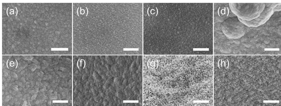
**Figure S2** (a-d) SEM image of NiWO<sub>4</sub>/Ni foam with different reaction time: (a) 4 h, (b) 6 h, (c) 10 h, (d) 12 h; (e-h) SEM image of CoWO<sub>4</sub>/Ni foam with different reaction time: (e) 4 h, (f) 6 h, (g) 10 h, (h) 12 h (Scale bar: 500 nm).
