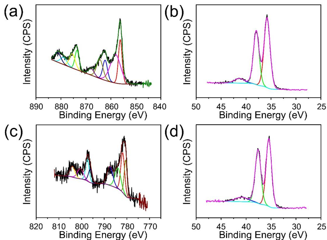
**Figure S5** (a) Ni<sup>2p</sup> XPS spectrum and (b) W<sup>4f</sup> XPS spectrum of NiWO<sub>4</sub> nanostructures; (c) Co<sup>2p</sup> XPS spectrum and (d) W<sup>4f</sup> XPS spectrum of CoWO<sub>4</sub>
