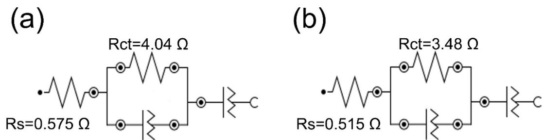
**Figure S7** the equivalent fitting circuit of NiWO<sub>4</sub>/Ni foam and CoWO<sub>4</sub>/Ni foam.
