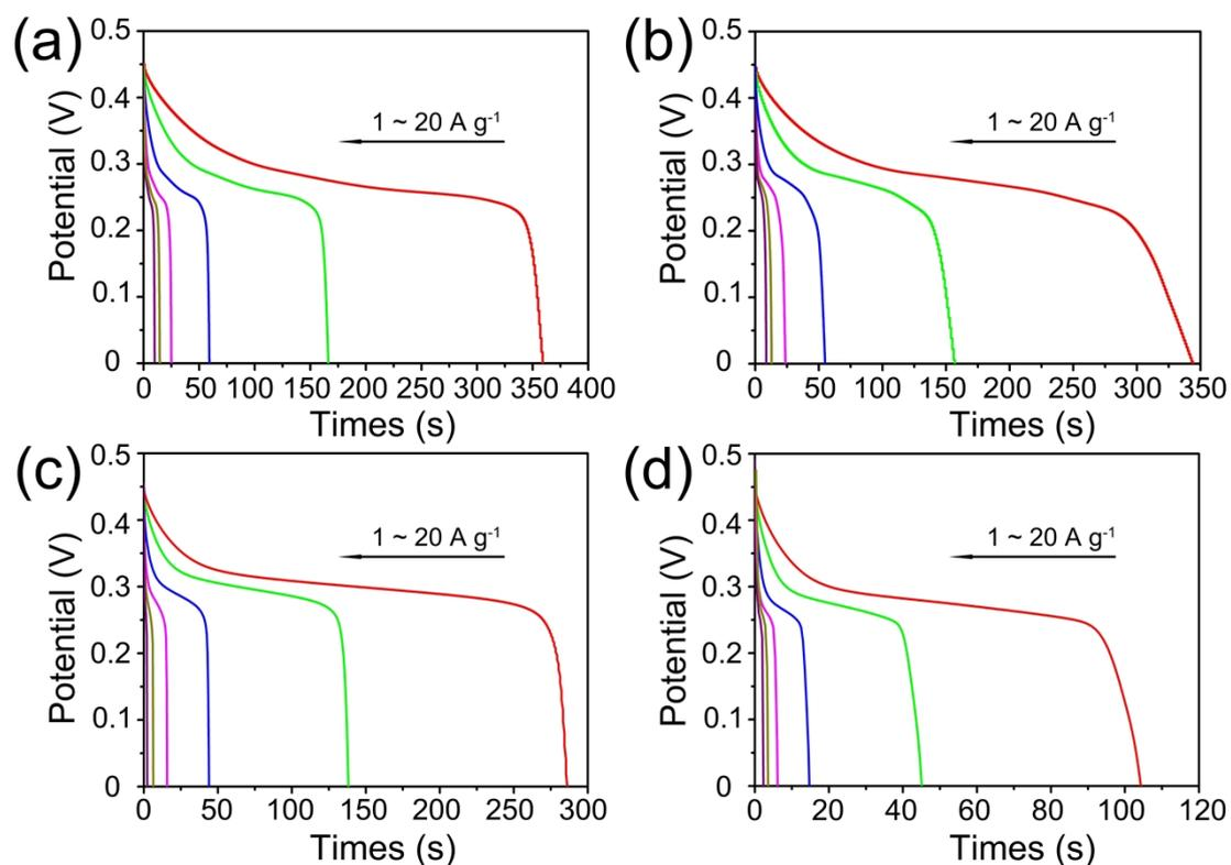
**Figure S6** Discharge curves of (a) NiWO<sub>4</sub>/Ni foam nanostructures, (b) CoWO<sub>4</sub>/Ni foam nanostructures, (c) NiWO<sub>4</sub> powders, (d) CoWO<sub>4</sub> powders at the current densities of 1, 2, 5, 10, 15, 20 A g<sup>-1</sup> respectively.
