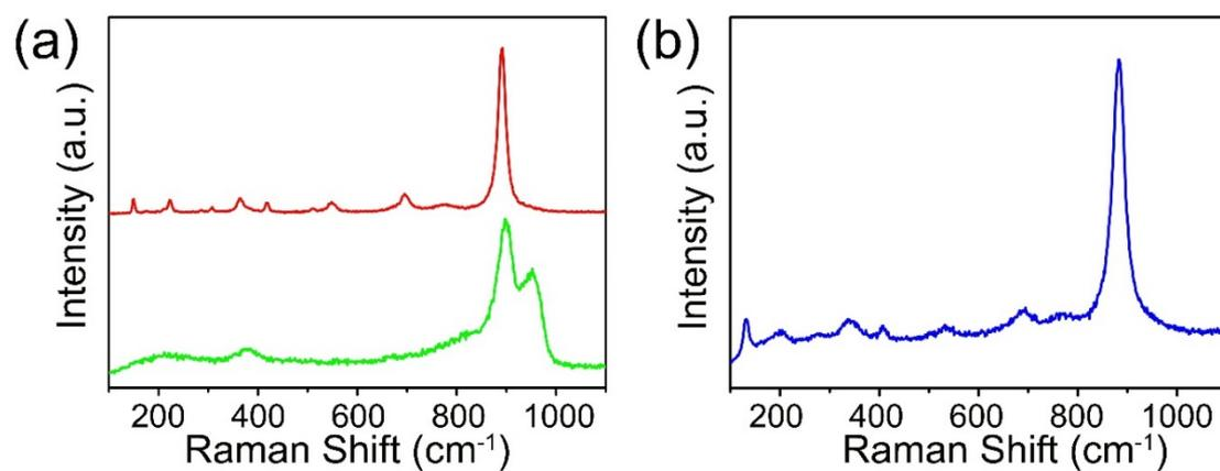
after (red line) annealing; (b) Raman spectrum of CoWO<sub>4</sub> nanostructures.
