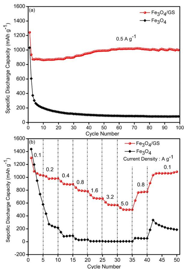
**Figure S3** the test electrode is prepared with a weight ratio of 80:10:10 for active material, acetylene black and binder, respectively. Cycling performance (a) 0.5 A g<sup>-1</sup> and Rate Capability (b) at various current densities are shown.
