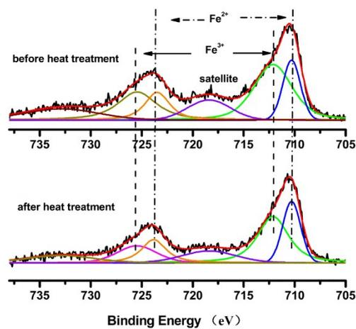
Figure S1. Fe 2p XPS spectra of Fe<sub>3</sub>O<sub>4</sub>/GS before and after heat treatment
