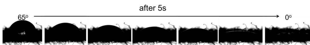
Fig. S4 Change of the water contact angle of the pristine fabric with the drop ages.
