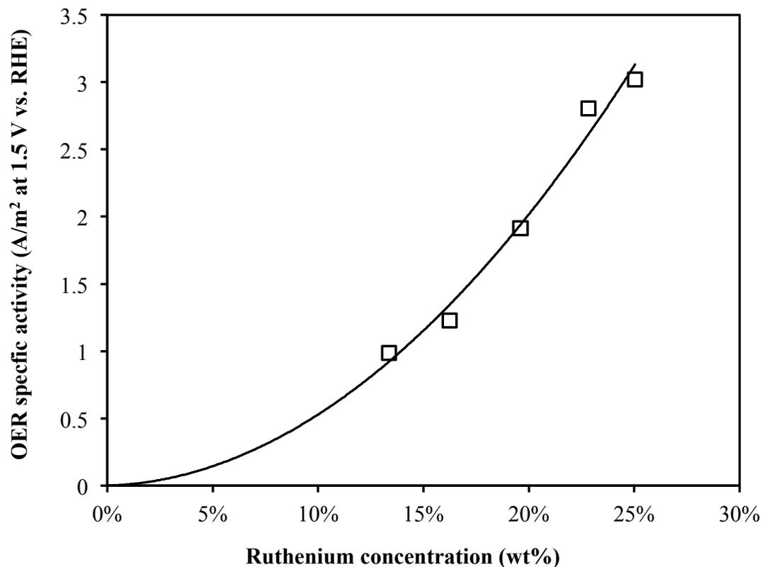
**Figure S6.** Specific OER activities (at 1.5 V vs. RHE) for lead ruthenate pyrochlores with varying ruthenium concentrations ( $\text{Pb}_{2+x}\text{Ru}_{2-x}\text{O}_{6.5}$ ;  $x = 0, 0.3, 0.5, 0.7$  and  $0.9$ ). Activities calculated from capacity-corrected positive-going scans at  $5 \text{ mV s}^{-1}$  in  $0.1 \text{ M KOH}$ .
