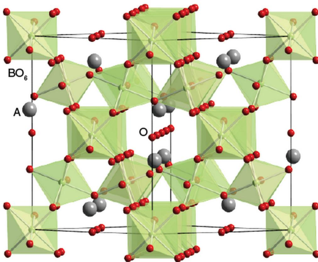
**Figure S1.** Crystalline structure of pyrochlores with general formula  $A_2B_2O_{7-y}$ .<sup>1</sup>
