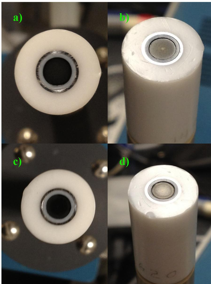
**Figure S5.** Typical appearance of the catalyst deposited onto the surface of the GC electrode before starting the OER experiment (a and b), and same electrode after the experiment was done (c and d). Pictures show a complete covered GC substrate and a smooth and uniform electrode; no degradation or partial disintegration of the electrode was observed after running the OER experiment.
