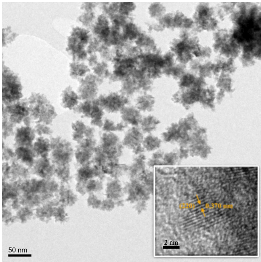
**Figure S2.** TEM micrograph of  $\text{Pb}_2\text{Ru}_2\text{O}_{6.5}$ . The material showed particle-like aggregates of approximately 50-100 nm constituted of smaller particles glued together. The insert in the figure shows the Fresnel fringes for a particle demonstrating that some particles were crystalline.
