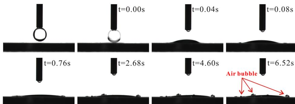
**Figure S6.** Time sequence of an oil droplet contacting the laser-induced surface in water after dark storage. The oil droplet spreads out quickly once it contacts the substrate, showing underwater superoleophilicity. In addition, some air bubbles appear on the oil liquid surface as the oil droplet spreads.
