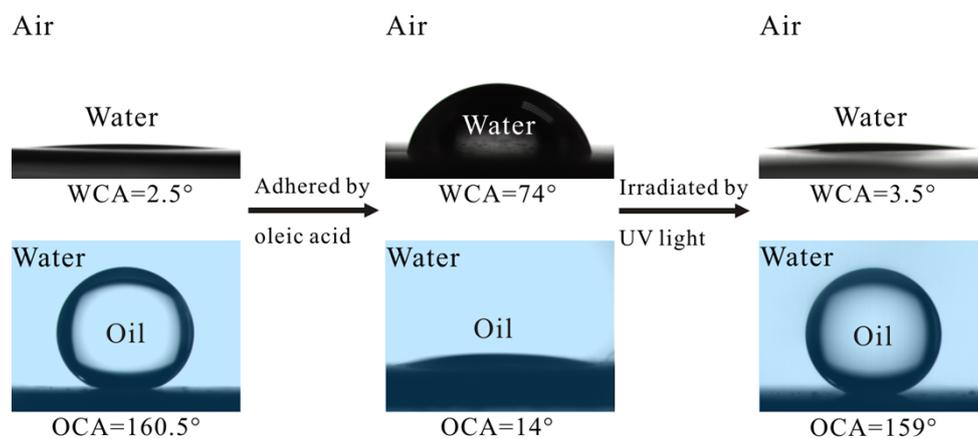
**Figure S5.** WCAs and underwater OCAs of the sample after being adhered by oleic acid and subsequently irradiated by UV light, indicating good antifouling property of the femtosecond laser-induced TiO<sub>2</sub> surface under UV light irradiation.
