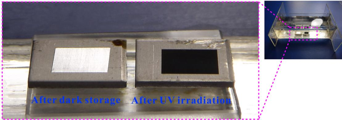
**Figure S2.** Femtosecond laser ablated Ti samples in water. A silver mirror can be seen for the laser-induced region after dark storage, but the mirror does not appear for the sample after UV irradiation.
