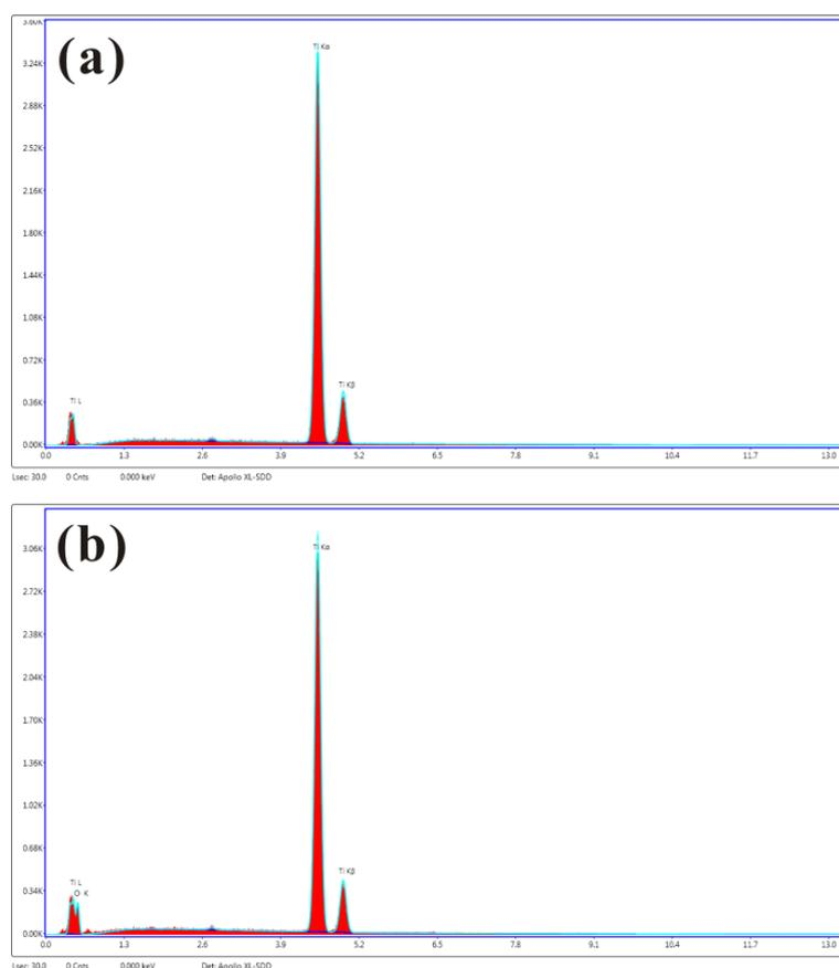
**Figure S1.** Complete EDXS results of the Ti surface before (a) and after (b) femtosecond laser ablation.
