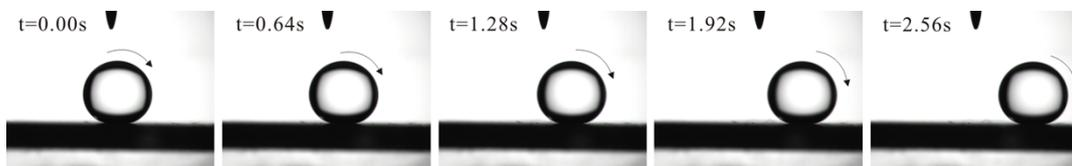
**Figure S3.** Images of an oil droplet rolling off on a UV-irradiated microstructured surface in water tilted at  $1^\circ$ .
