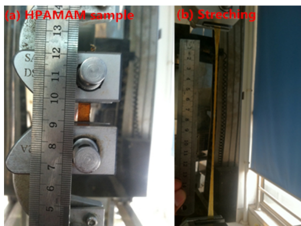
Fig. S5 (a) HPAMAM sample in original state: the gauge was 10 mm; (b) HPAMAM sample was extended to a length more than 150 mm
