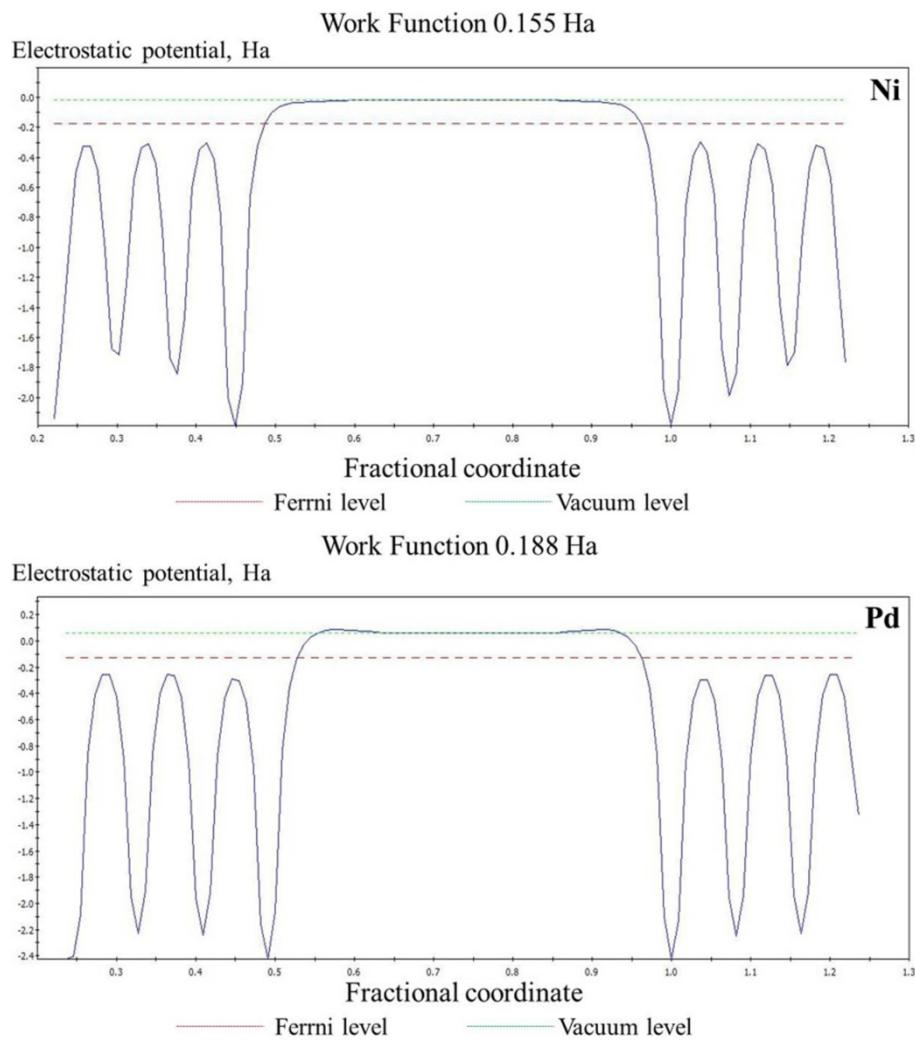
**Figure S6.** The calculated work functions for Ni (111) and Pd (111) surfaces (1Ha=27.212eV).
