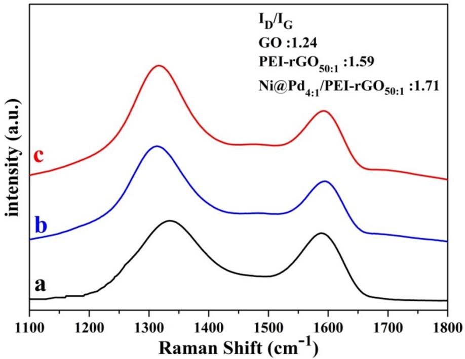
**Fig. S4** Raman spectra of (a) GO; (b) PEI-rGO<sub>50:1</sub> and (c) Ni@Pd<sub>4:1</sub>/PEI-rGO<sub>50:1</sub>.
