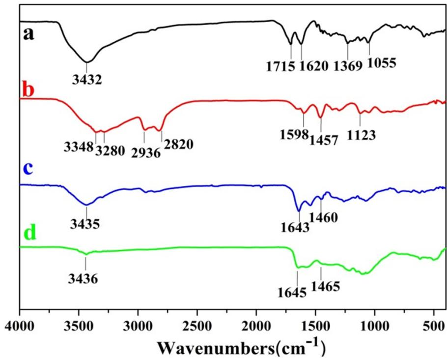
**Fig. S3** FT-IR spectra of (a) GO; (b) PEI; (c) PEI-rGO<sub>50:1</sub>; and (d) Ni@Pd<sub>4:1</sub>/PEI-rGO<sub>50:1</sub>.
