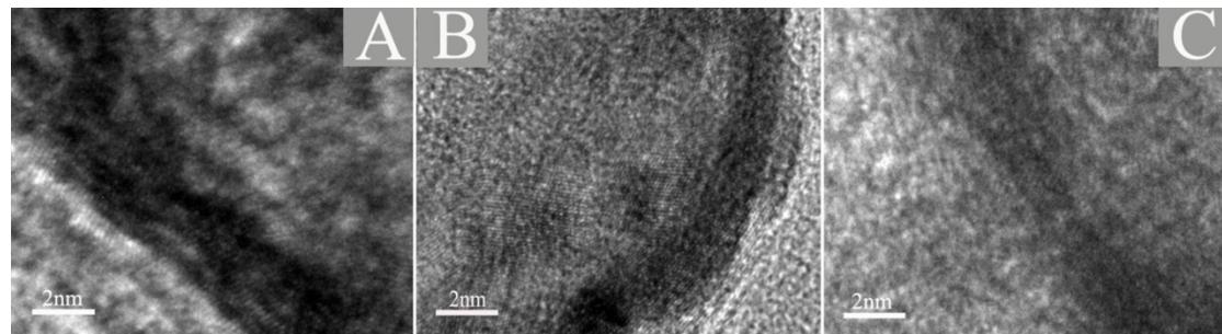
**Fig. S1** HRTEM images of Pd shell thickness of (A) Ni@Pd<sub>3:1</sub> hybrids; (B) Ni@Pd<sub>4:1</sub> hybrids; (C) Ni@Pd<sub>5:1</sub> hybrids.
