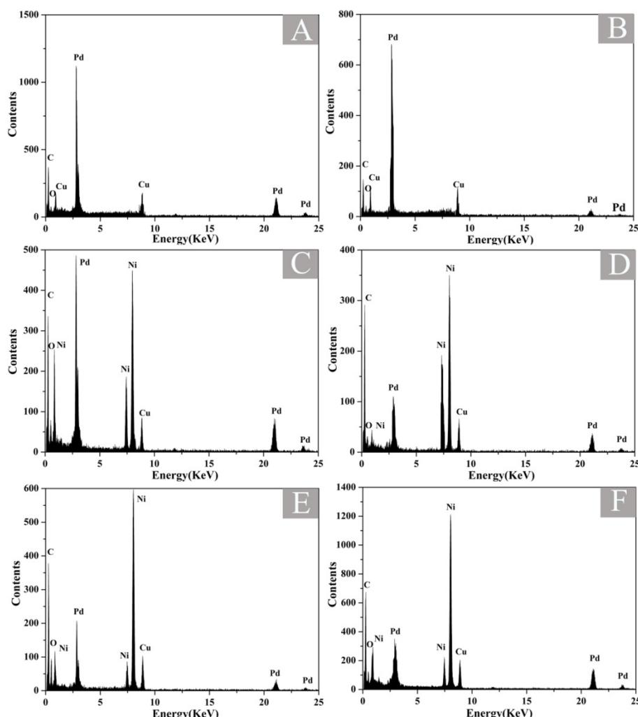
**Fig. S2** EDX spectrum of (A) Pd<sub>hollow-1</sub> hybrids; (B) Pd<sub>hollow-2</sub> hybrids; (C) Ni@Pd<sub>2:1</sub> hybrids ; (D) Ni@Pd<sub>3:1</sub> hybrids; (E) Ni@Pd<sub>4:1</sub> hybrids; (F) Ni@Pd<sub>5:1</sub> hybrids.
