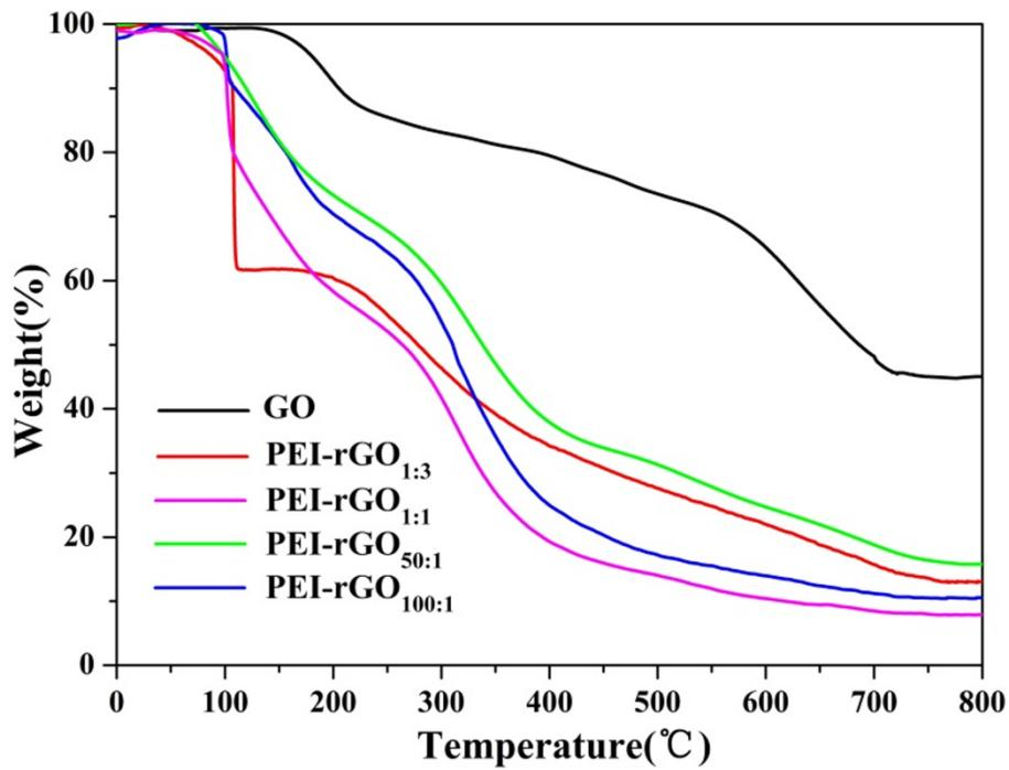
**Fig. S5** TGA curves of GO, PEI-rGO<sub>1:3</sub>, PEI-rGO<sub>1:1</sub>, PEI-rGO<sub>50:1</sub>, PEI-rGO<sub>100:1</sub>.
