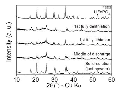
S.1 XRD patterns of bare LiFePO<sub>4</sub> nanoparticle. And XRD patterns of SS nanoparticle and its fully delithiated and lithiated and state of discharge 50% electrode.
