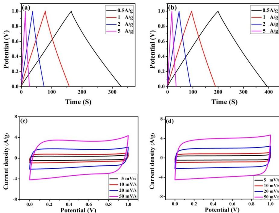
**Fig.S3** Galvanostatic charge-discharge curves of GCA/CNT-S (a) and GCA/CNT-L (b) measured at different current density; Cyclic voltammograms measured at different scan rate of GCA/CNT-S (c) and GCA/CNT-L (d).
