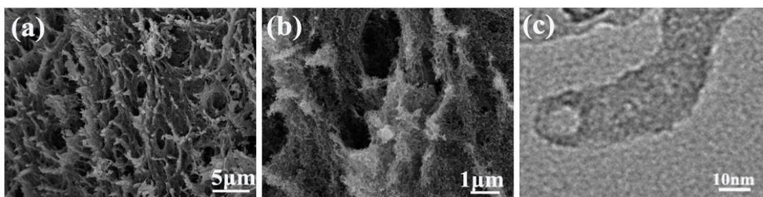
Fig.S1 SEM images of GCA/CNT (a, b); TEM image of GCA/CNT (c)
