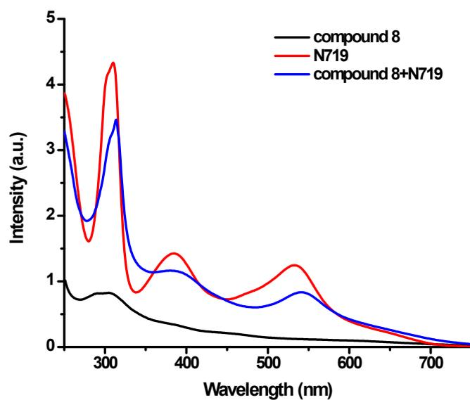
Fig. S8. UV-Vis absorption spectra of compound **8** in  $\text{CHCl}_3$ , **N719** and compound **8+N719** in mix solution of acetonitrile and n-butyl alcohol ( $v/v=1:1$ ).
