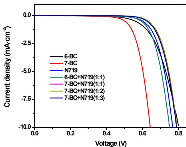
Fig.S11 Dark current- voltage curves of DSSCs devices based on **6-BC**, **7-BC**, **N719**, **6-BC+N719(1:1)**, **7-BC+N719(1:1, 1:2, 1:3)**
