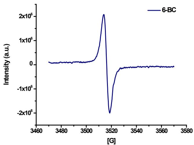
Fig. S7. EPR spectrum of **6-BC** in  $\text{CHCl}_3$ .
