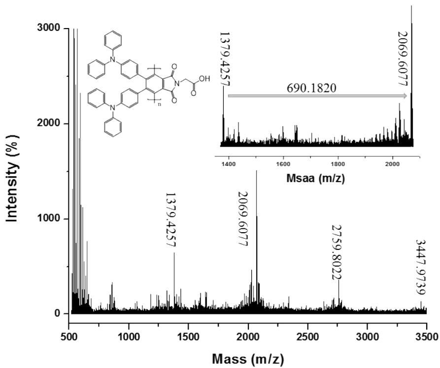
Fig.S6 MALDI-TOF mass spectrum of the oligomer part of 6-BC.
