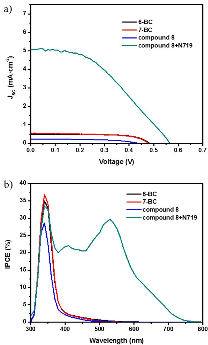
Fig.S10 a) J-V curves and b) IPCE spectra of DSSCs sensitized with **6-BC**, **7-BC**, compound **8** and compound **8+N719**.
