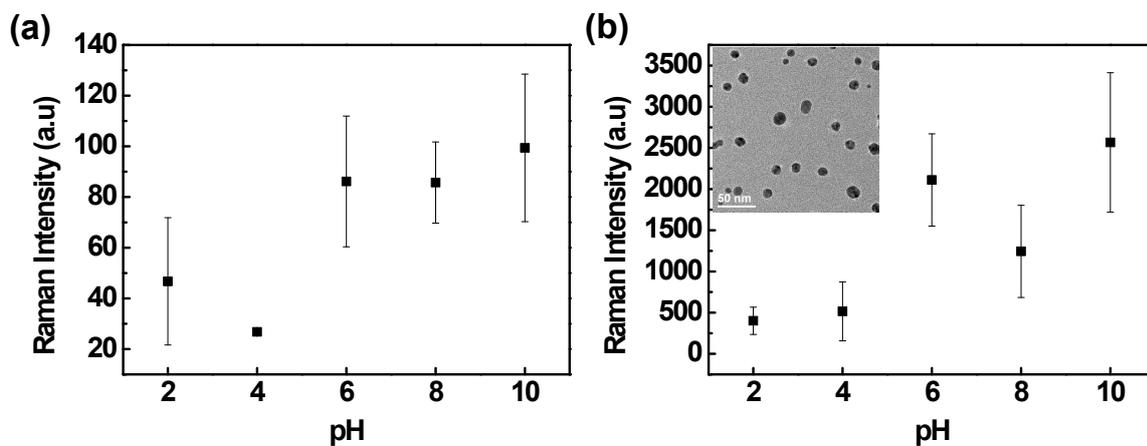
**Figure S7.** Raman intensity plots for S4VP@Ag monolayer films fabricated by (a) S4VP (31k) and (b) S2VP (265k) without BT target molecule. A ring stretching mode ( $1602\text{ cm}^{-1}$ ) of a P4VP block was plotted, instead of characteristic wavelength of benzenethiol (BT) molecules.
