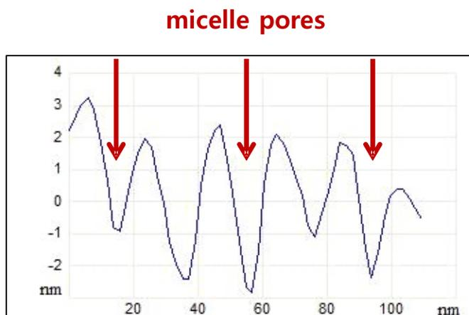
**Figure S3.** Cross-sectional line profile of S4VP@Ag monolayer film on Si substrate at pH = 10. Cross-sectional line profile was obtained from white dotted line in left AFM image, indicating small pores in the center of each micelle.
