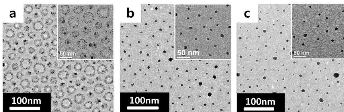
**Figure S1.** TEM images of S4VP@Ag monolayer micellar film with relatively small P4VP block ratio at (a) pH = 2, (b) as-prepared (pH = 7), and (c) pH = 10.
