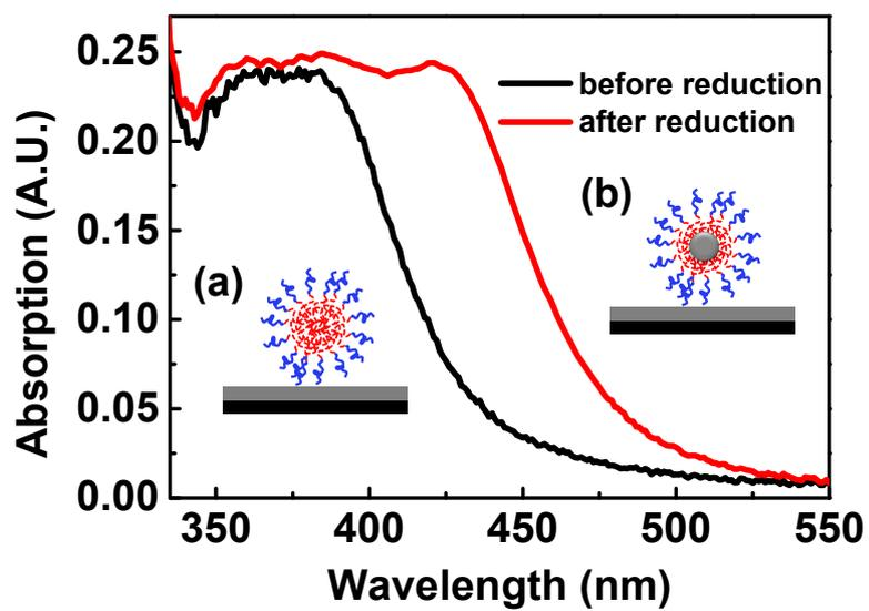
Figure S4. UV-vis absorption spectra of as-prepared S4VP micelles on Ag film for comparison of (a) before and (b) after reduction. The localized surface plasmon of Ag NP shows at 430 nm wavelength with S4VP resonance peak.
