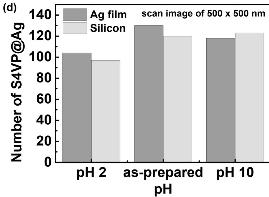
**Figure S6.** AFM images of S4VP@Ag monolayer film on Ag substrate at (a) pH = 2, (b) as-prepared (pH = 7), and (c) pH = 10. (d) These surface density of S4VP@Ag on Ag and Si substrates are plotted by bar graph based on AFM images. All surface morphologies in different pH conditions are almost same for Si substrate.
