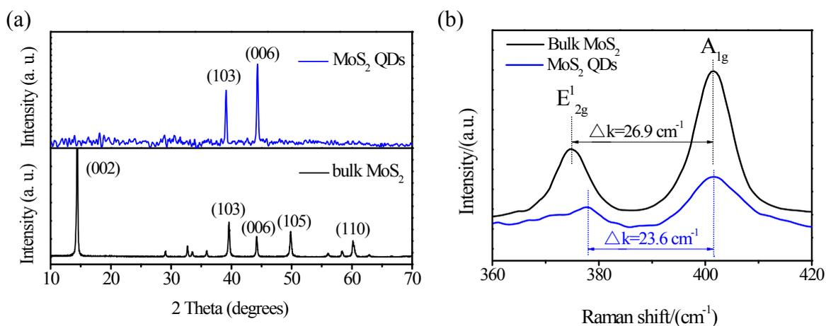
**Fig. S2.** (a) XRD patterns of MoS<sub>2</sub> QDs and bulk MoS<sub>2</sub>. (b) Raman spectra recorded using a 532 nm laser for MoS<sub>2</sub> QDs and bulk MoS<sub>2</sub>.
