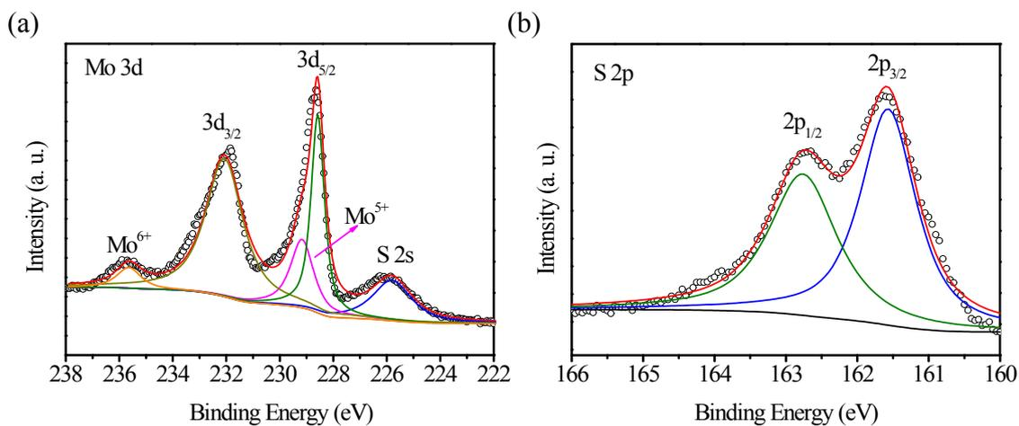
**Fig. S1.** High-resolution XPS of (a) Mo 3d and (b) S2p spectra of the MoS<sub>2</sub> QDs.
