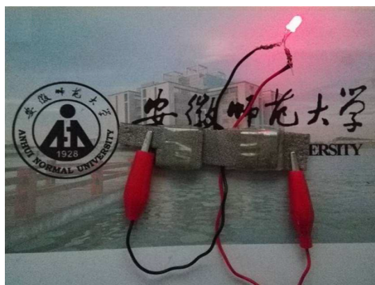
Figure S7. Photograph of a red LED lighted up by two \text{NiCo}_2\text{S}_4/\text{C} devices in series.
